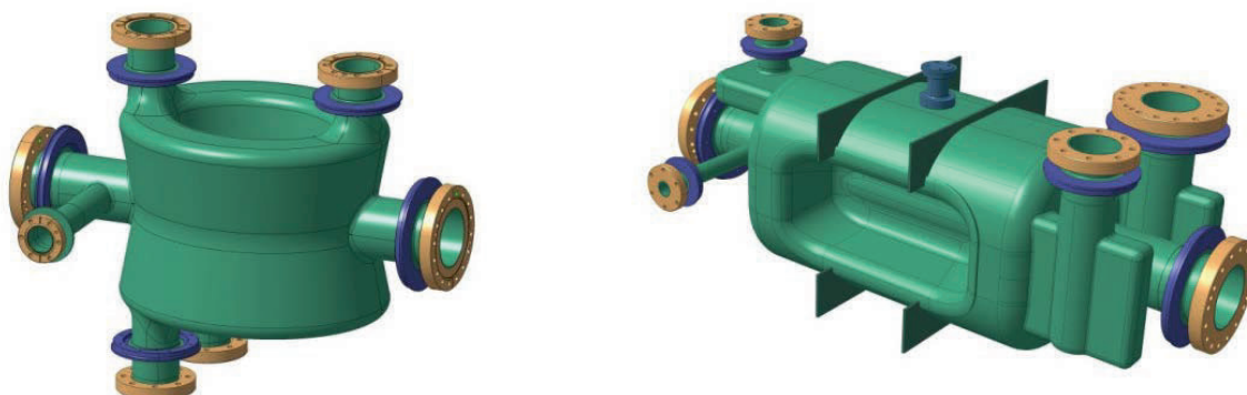
Figure 4-8: Schematic view of the cavity with interfaces (left) DQW; (right) RFD.
