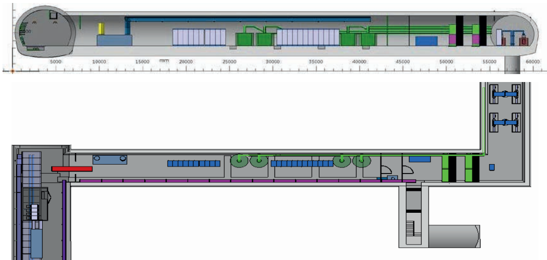
Figure 4-23: Schematic of the RF system layout (four per IP side) in the underground cavern above the LHC tunnel lateral view (top); and top view (bottom); Note that these are only estimated values of space requirements.
