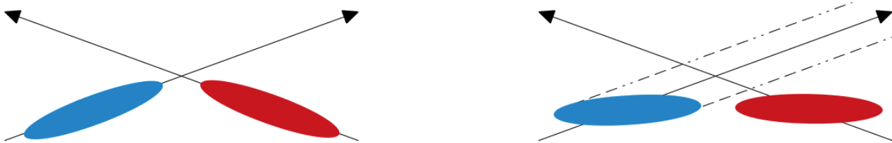
Figure 4-1: Bunches colliding with a crossing angle without crab crossing (left); with the crab crossing (right).
