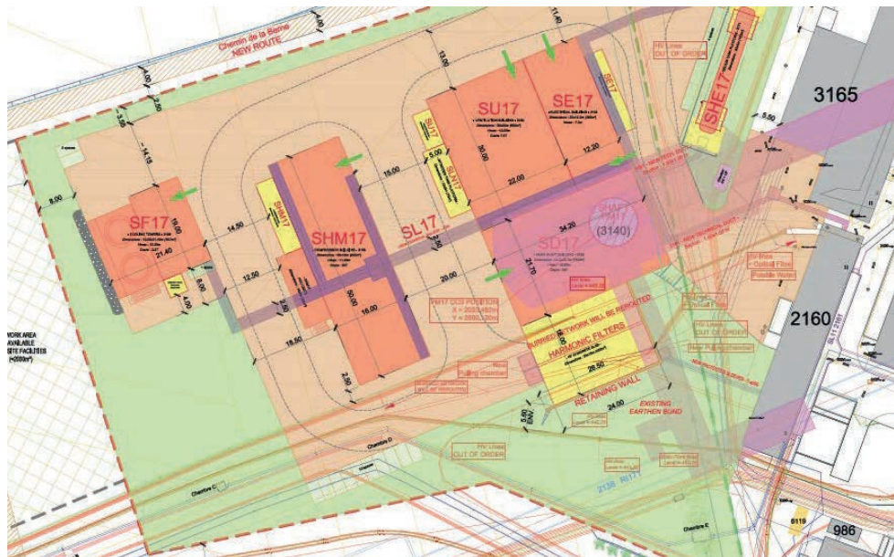
Figure 15-11: The LHC Point 1 with the new HL-LHC surface building.
