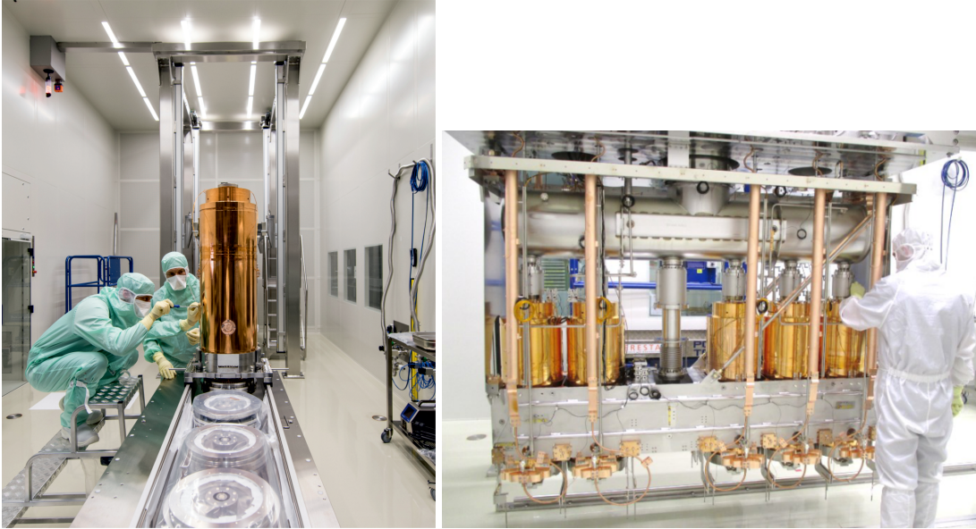
(a) Installation of instrumentation on the rinsed superconductive cavity before assembly into CM1. (b) Final verifications on CM2 before closure and transport to the ISOLDE facility.
