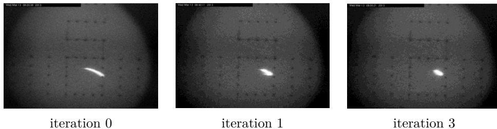
Figure 8.10: Phosphorous beam profile monitor measurements at the end of the FACET linac, before the dispersion correction, after one iteration step, and after three iteration steps. Iteration zero is before the correction.
