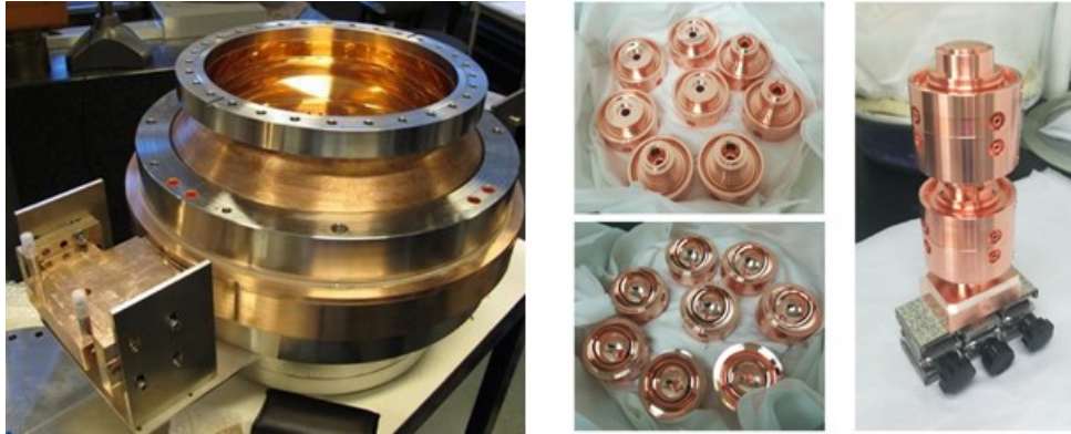
Figure 5.9: C-band BOC fabricated at PSI shown is left. CCC cavities half shells and one of four assembled CCC cavities doublet are shown right.
