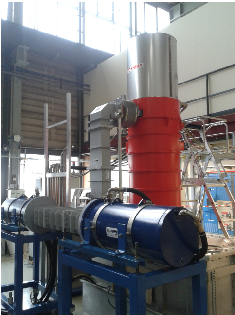
Figure 5.10: Left: The 1 GHz klystron test stand at CERN with the Toshiba klystron installed; Right: Efficiency, Output power and gain as a function of voltage for the Toshiba MBK.
