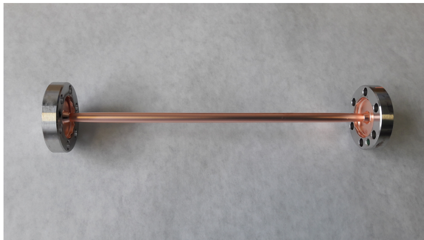
Figure 5.21: Electroformed copper chamber integrating stainless steel flanges.
