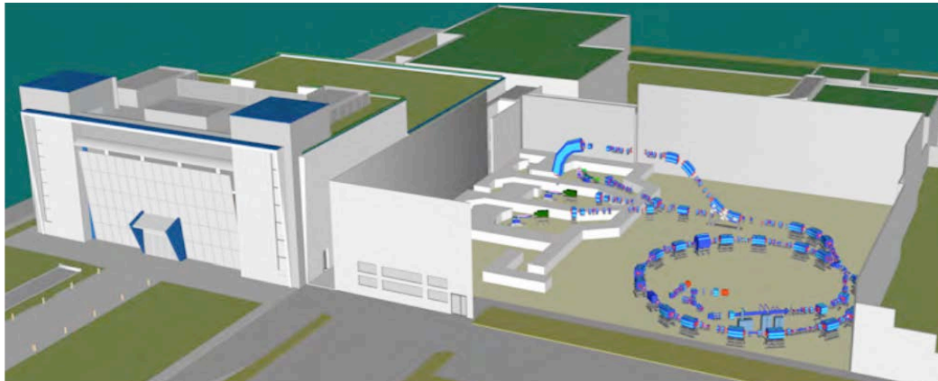
Fig. 10: Perspective view of the CNAO centre, which features 3 treatment rooms with 4 therapeutic beams (3 horizontal and 1 vertical), and 1 experimental room (not represented).
