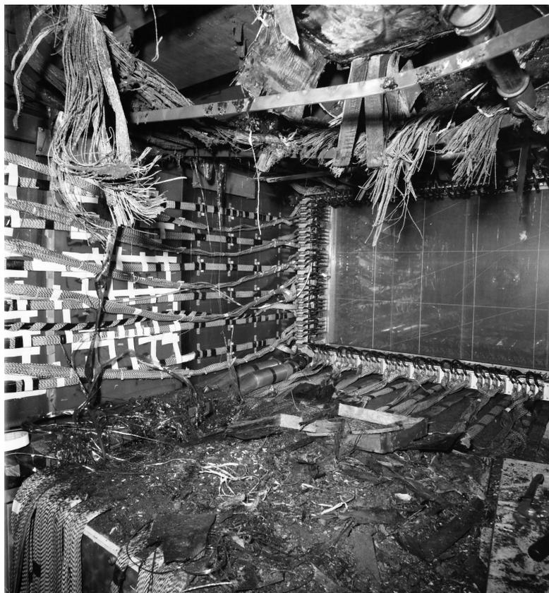
**Fig. E.1:** The effects of the fire inside the Forward Spectrometer magnet (image credit CERN, [CERN-PHOTO-1825941](https://cds.cern.ch/record/1825941))
