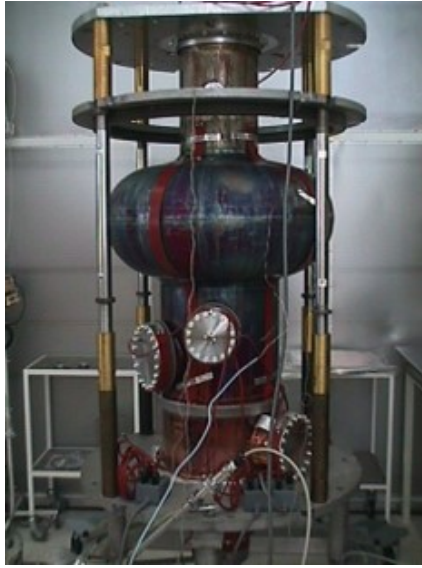
Fig. II.5.34: LHC cavity after Nb thin film coating by sputtering (Image courtesy of CERN).
