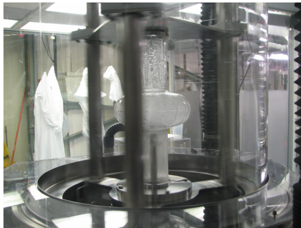
Fig. II.5.67: Demonstrating HPWR in a test transparent plastic cavity [46].
