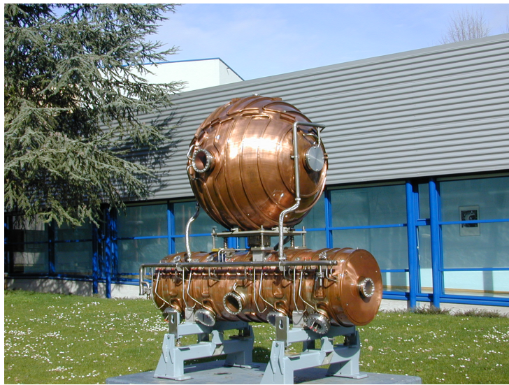
Fig. II.5.1: Normal conducting CERN LEP cavity with a spherically-shaped storage cavity on top [2].
