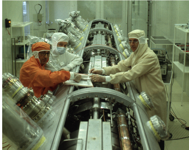
Fig. II.5.66: Clean room preparation on one of the superconducting cavities for the LEP-2 upgrade [45].
