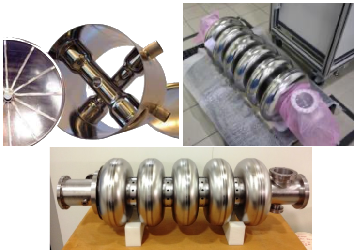
Fig. II.5.38: The three different ESS cavity families: low-beta \beta = 0.5 two-spoke cavity (top left, courtesy IJC Lab), the 6-cell elliptical medium-beta \beta = 0.67 cavity (top right, courtesy INFN-LASA, and the 5-cell elliptical high-beta \beta = 0.86 cavity (bottom, courtesy CEA).
