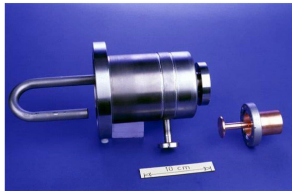
Fig. II.5.B.4: LHC coupling loop for a HOM damper [55].
