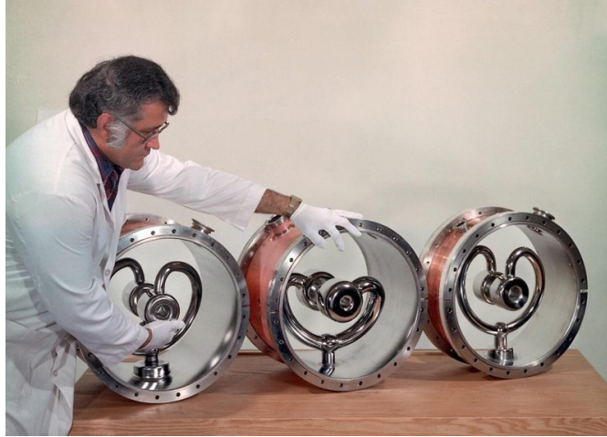
Fig. II.5.39: Spiral resonator SRF cavities from ATLAS-ANL (note the lead plating inside the cavity copper body) [28].
