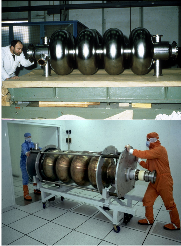
Fig. II.5.30: Top: bulk niobium cavity of LEP [23]. Bottom: niobium-coated copper prototype (Image courtesy of CERN).
