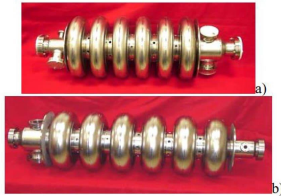
Fig. II.5.37: The SNS \beta = 0.61 and \beta = 0.81 cavities [27].
