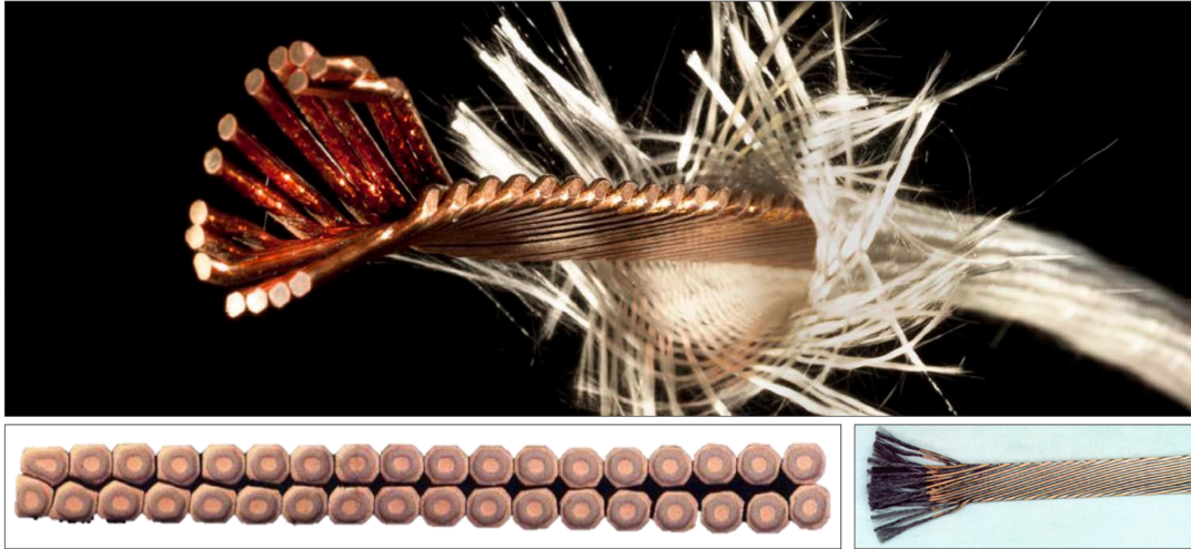
Fig. II.6.23: Images of a multi-strand Rutherford cable.
