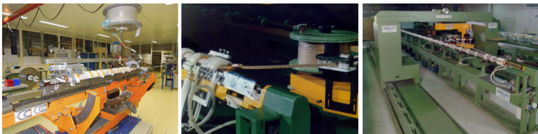
Fig. II.6.51: Left: winding machine for short coils with a rotating mandrel. Centre and right: winding machine for long coils.
