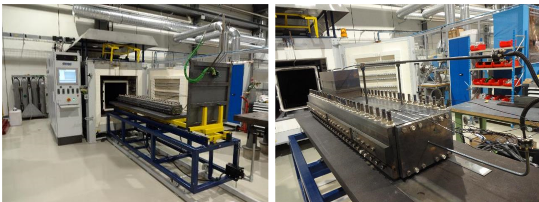
Fig. II.6.55: Reaction fixture inserted in a reaction oven (CERN MQXF5 coils).
