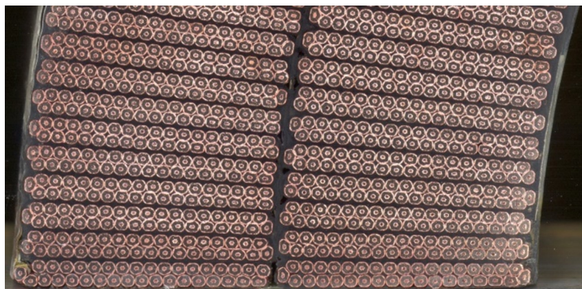
Fig. II.6.30: Cross-section of a superconducting coil.
