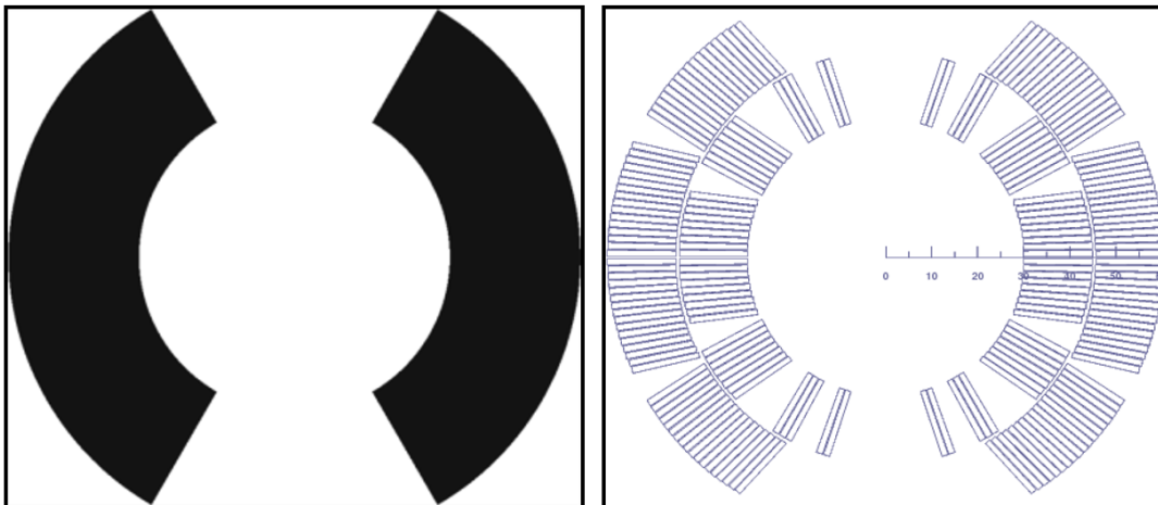
Fig. II.6.34: Cross section of a sector coil (left) and the positioning of Rutherford cables in the sector for a “real” \cos\theta coil (right).
