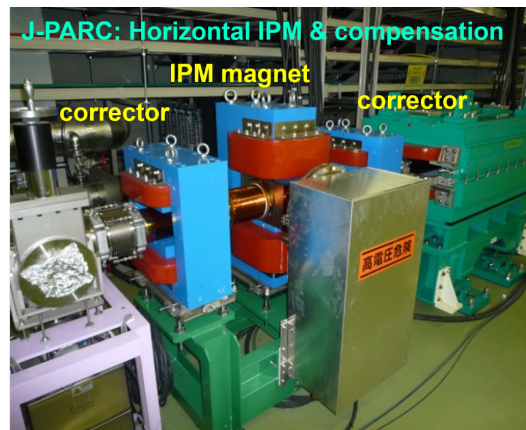
Fig. II.9.62: Left: Schematic trajectory of an ion beam within the main IPM magnet field and the two corrector fields. Right: A photo of the J-PARC IPM realization with a main magnet for the horizontal profile and two corrector dipoles; the dipole field is B = 250 mT with a gap of d_{gap} = 220 mm, see [74].
