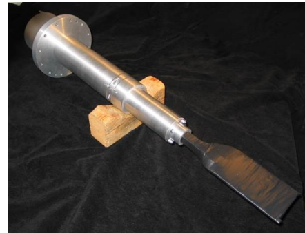
Fig. II.9.32: Left: The scheme of a plastic scintillation counter connected to the photo-multiplier via a plastic light guide. Right: Photo of scintillator wrapped in black tape. The photomultiplier and its base is inside of the metal housing.
