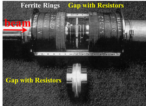
Fig. II.9.137: Photo of the wall current monitor used at Fermilab for protons, from [169]. The ceramic gap is shown separately. The ferrite rings and the printed circuit with the resistors are visible.
