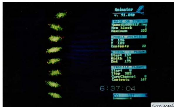
Fig. 10: Head–tail mode m = 1 , observed in the Large Electron–Positron Collider. Screen shot with streak camera
