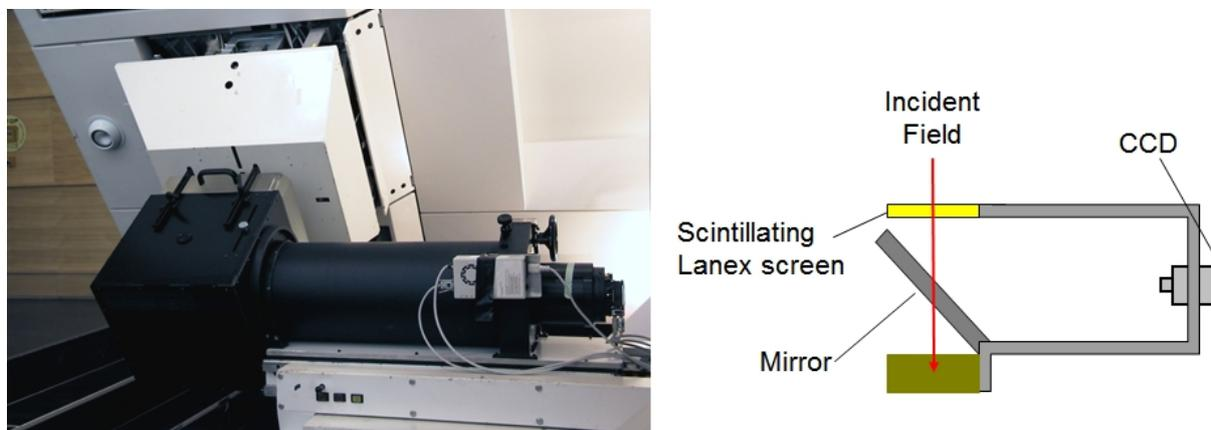
**Fig. 6:** Scintillating-CCD dosimetry system at PSI Gantry 1 (left) and a schematic representation (right)
