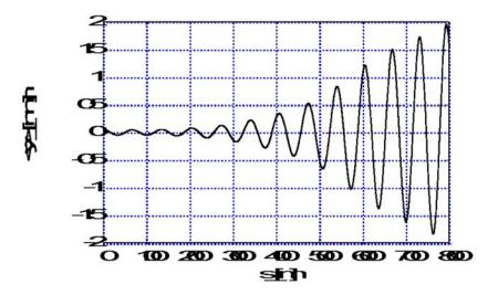
Fig. 7: HOMDYN [20] simulation of a typical BBU instability, 50 µm initial offset, no energy spread
