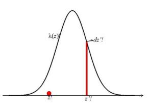
**Fig. 6:** Convolution integral for a charge distribution to obtain the energy loss of a particle due to the whole bunch Equation (26) allows us to define the longitudinal wake potential of a distribution:
