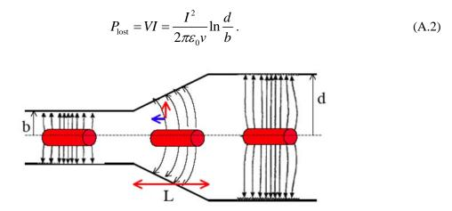
Fig. A.2: Smooth transition of length L (taper) from a beam pipe of radius b to a larger beam pipe of radius d
