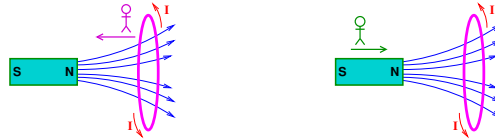
Fig. 4: Effect of relative motion of a magnetic field and a conducting coil, observed from a co-moving and the rest frame.
