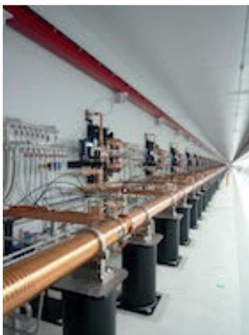
**Fig. 74:** SACLA C-band linac
