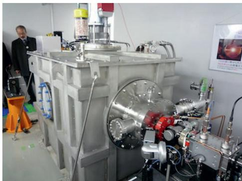
**Fig. 71:** Thermoionic gun of SCSS Test Accelerator, with T. Shintake
