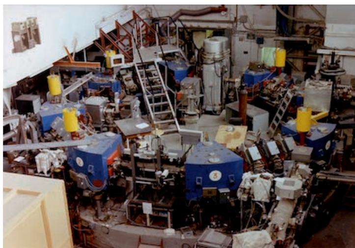
**Fig. 36:** ACO storage ring used for the second world wide FEL in Orsay (France), dipoles in blue
