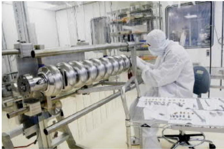
Fig. 35: Cavities during the assembly process in a clean room
