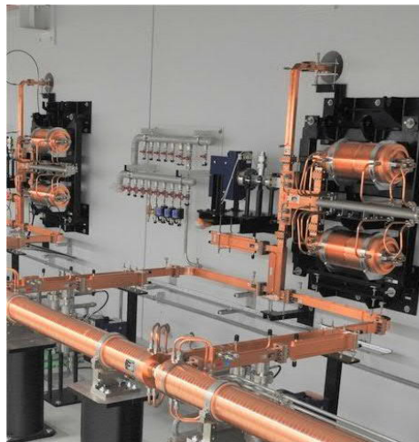
Fig. 54: Picture of the C-band SLED system implemented at Spring 8 [13, 14]
