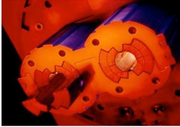
**Fig. 2:** Superconducting dipole magnet in the LHC storage ring
