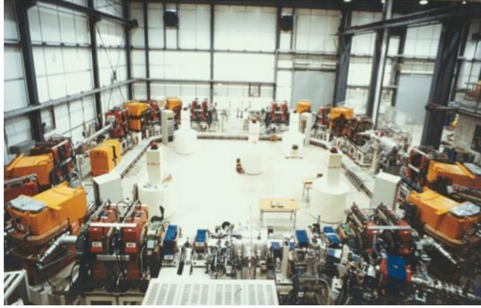
**Fig. 5:** The TSR storage ring, Heidelberg, is a typical example of a separate-function strongly focusing storage ring [4].
