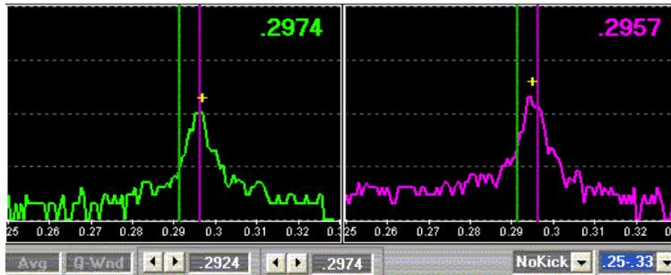
**Fig. 13:** Tune signal of proton beam in storage ring (HERA-p)
