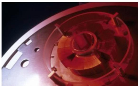
**Fig. 4:** Superconducting quadrupole magnet in the LHC storage ring
