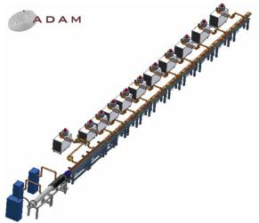
**Fig. 17:** Layout of a high-frequency linac for proton therapy, proposed by the CERN spin-off company A.D.A.M. (courtesy of A.D.A.M.).
