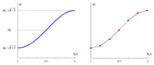
**Fig. 4:** Dispersion curve for coupled cavity oscillators with coupling factor *k*. In the case of TW mode (left), the dispersion curve is continuous (blue line), while for SW mode, only some modes are allowed (red dots).
