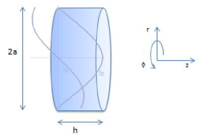
Fig. 5: Pillbox cavity, with longitudinal electric and azimuthal magnetic field components
