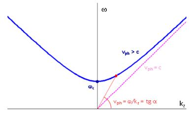
Fig. 1: Dispersion relation of a waveguide system
