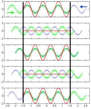
**Fig. 3:** Example of an SW pattern (red wave) obtained by superposition of two opposite travelling waves (blue and green curves). An SW cavity is obtained by inserting two metallic boundaries in correspondence of the two black lines.
