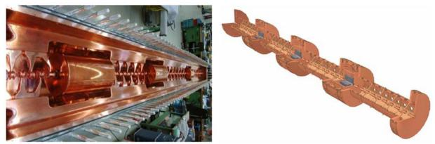
Fig. 11: Examples of IH (left) and CH (right) structures
