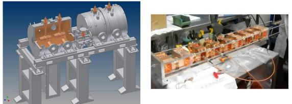
**Fig. 16:** Two examples of CCDTL structures: on the left is one of the 352 MHz SCDTL modules for LINAC4 (courtesy of M. Vretenar – CERN), and on the right is a 3 GHz SCDTL designed by ENEA for a proton therapy linac (courtesy of L. Picardi – ENEA).
