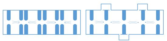
**Fig. 14:** Sketch of biperiodic CCL structures: on-axis-coupled structure (left) and side-coupled structure (right). The second case maximizes the space used for acceleration.
