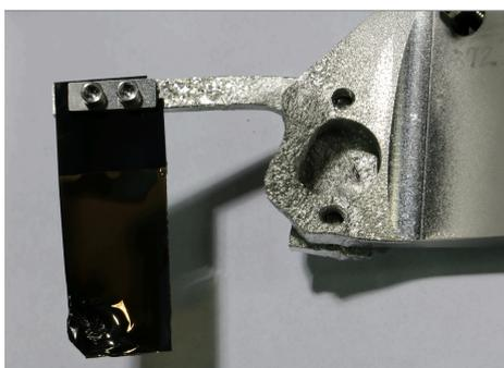
**Fig. 10:** Foil and bracket damaged by convoy electrons reflected back up from the catcher after 3 months of operation at 1.1–1.4 MW [11].
