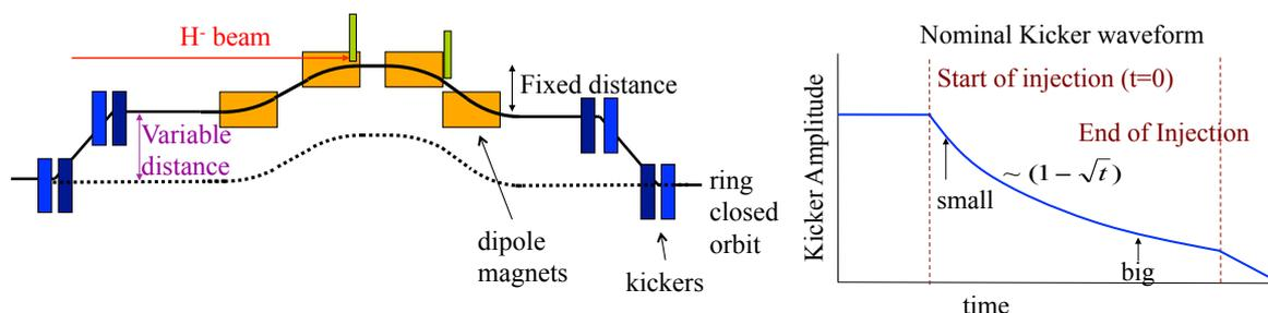
**Fig. 3:** Layout of the  $H^-$  charge exchange injection system used at SNS (left). Four dipoles (orange) are used to create the fixed injection chicane. Four horizontal and four vertical fast bumpers (light and dark blue) are powered with a current decaying in time proportionally to  $1 - \sqrt{t}$  (right) and provide a correlated transverse painting in both planes.
