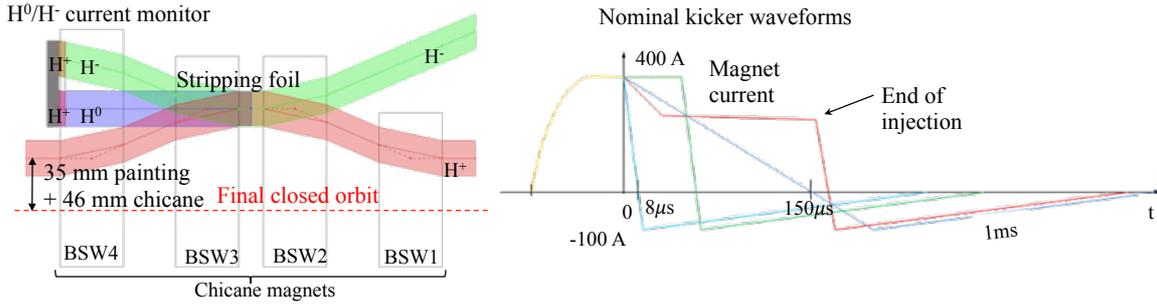
**Fig. 4:** Layout of the future  $H^-$  charge exchange injection system for the PSB (left). In this case, the injection bump is defined, only in the horizontal plane, by the chicane magnets and four kickers installed in the ring lattice. Different painting schemes can be obtained, by variable modulations of the current of the kickers, for the various users (right).
