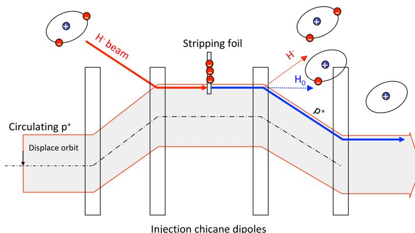
**Fig. 2:** Magnetic chicane installed around stripping foil. Varying the amplitude of the orbit bump during the injection process enables transverse phase space painting while avoiding excessive crossings, which might induce losses, foil heating, or emittance blow-up.
