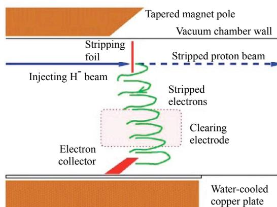
**Fig. 9:** The SNS stripping foil is installed inside one of the injection chicane magnets to drive the convoy electrons towards an electron catcher [13].
