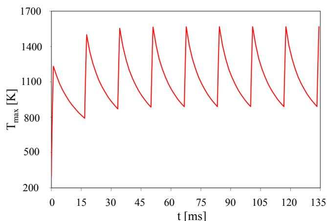
**Fig. 7:** Calculated temperature fluctuations at the SNS foil when operating with a 1 GeV, 1.5 MW beam
