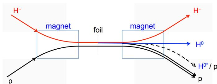
**Fig. 8:** Possible trajectories of  $H^{0*}$  atoms when they decay into  $p^+$ , owing to the effect of the magnetic field. If their trajectory is outside of the ring acceptance, these particles are lost [11].
