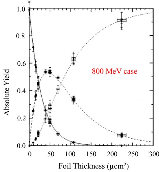
**Fig. 5:** Absolute yield of  $H^-$ ,  $H^0$ , and  $p^+$  as a function of the carbon foil thickness for an 800 MeV beam [10]
