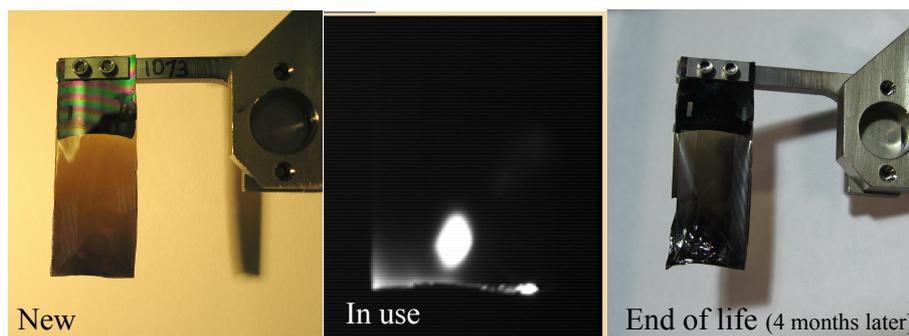
**Fig. 6:** Nanocrystalline diamond foil used at SNS when new, during, and after 4 months of operation
