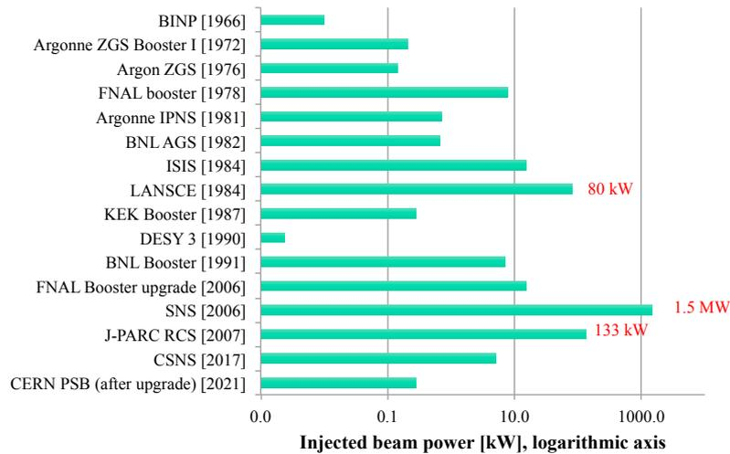
**Fig. 1:** Roadmap of the achieved and goal beam power for the main facilities using  $H^-$  charge exchange injection
