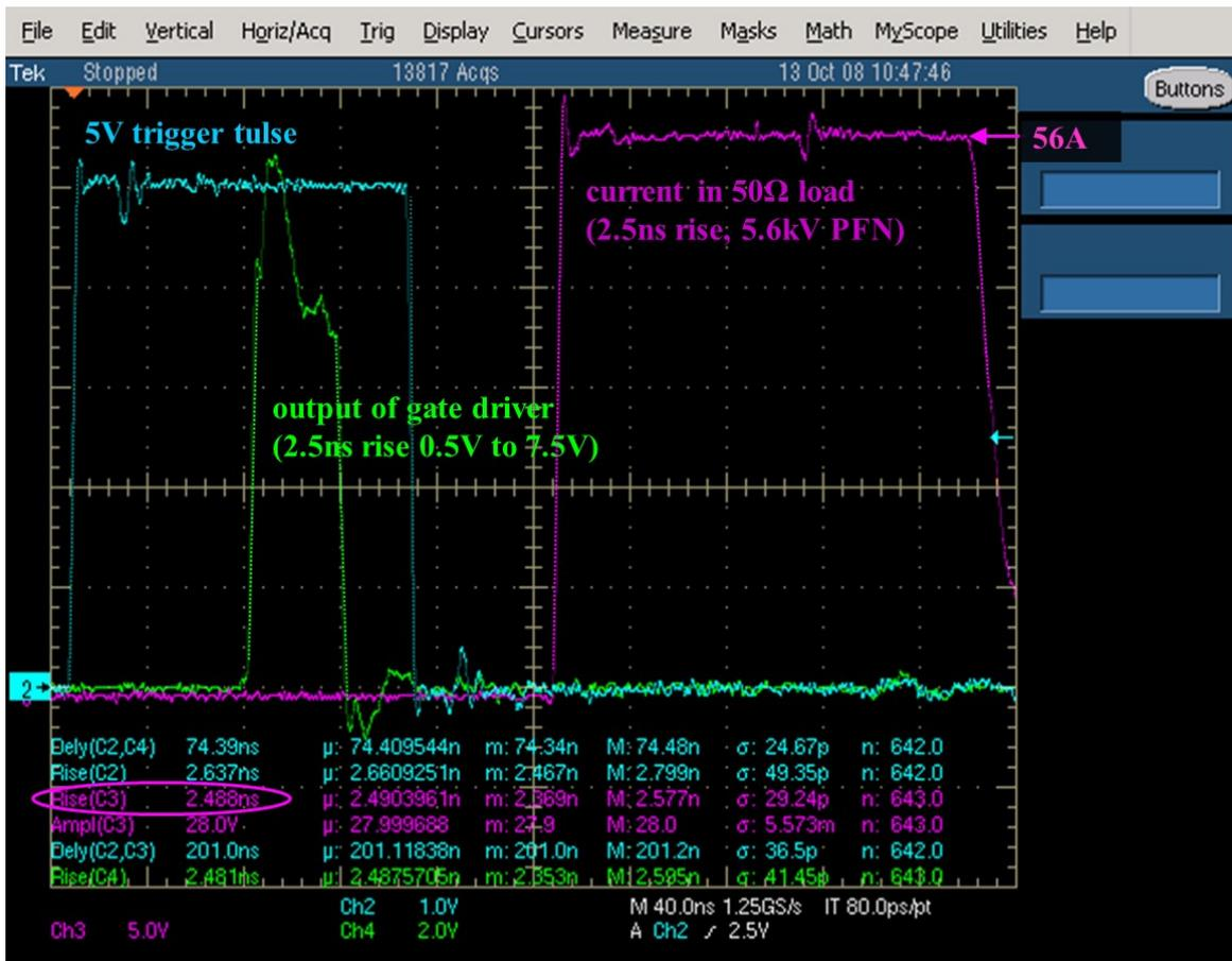
Fig. 44: Measured trigger pulse (cyan trace – 1 V/div), gate driver output (green trace – 2 V/div), and load current (lilac trace – 10 A/div) for a CTF3 tail-clipper kicker system.
