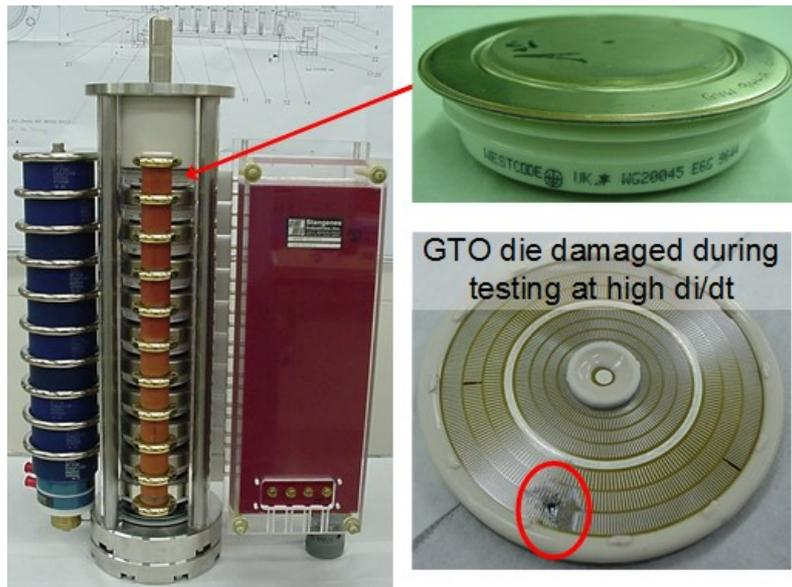
Fig. 24: Stack of-high power GTOs (LHS) and individual GTOs (RHS)
