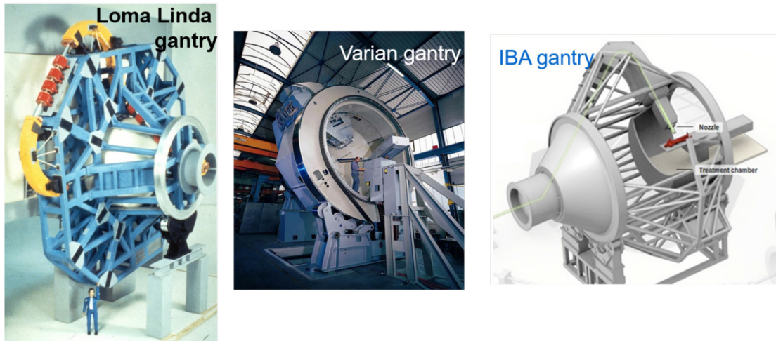
Fig. 8: Left—the ‘corkscrew’ gantry at Loma Linda; middle—the Varian gantry designed for scanning beams during its construction phase; and right—the IBA gantry.
