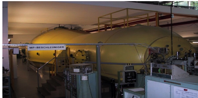
Fig. 26: Tandem Van de Graaff accelerator at the Max Planck Institute, Heidelberg
