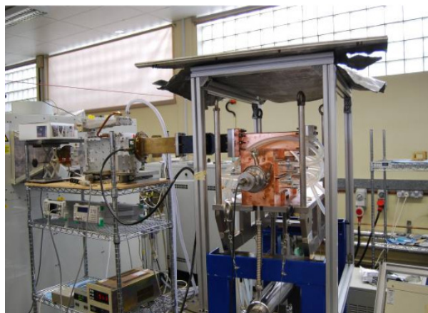
Fig. 10: The ACLIP module high-power RF test set
