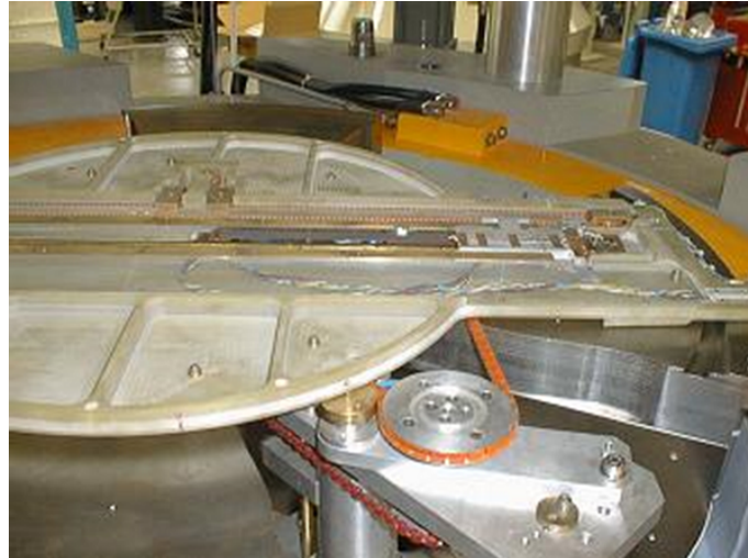
Fig. 16: Mapping system carrying a Hall probe that moves on a polar grid in the cyclotron median plane
