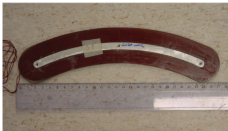
Fig. 55: Harmonic coil used in the IBA self-extracting cyclotron (note that the ruler measures centimeters)
