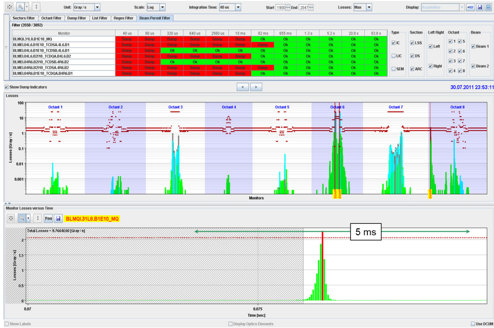
Fig. 22: Time structure of the beam losses caused by a UFO
