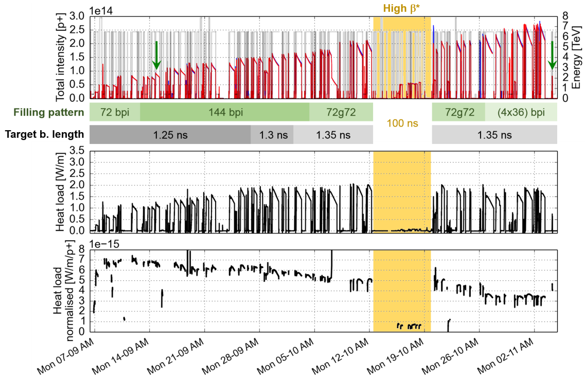
Fig. 14: Evolution of (top) beam intensity, (middle) average heat load in the arc magnets, and (bottom) heat load normalized to the beam intensity during the intensity ramp-up, with 25 ns beams
