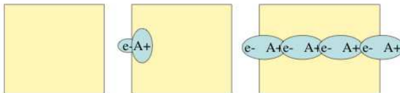
Fig. 19: Charge transfer in a dielectric medium, via a sequence of local polarizations
