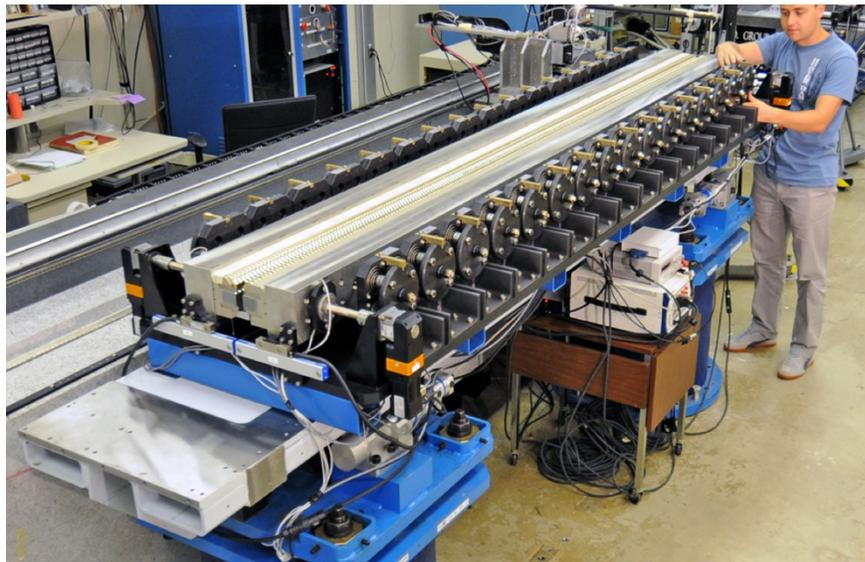
**Figure 11:** Prototype LCLS-II variable horizontal gap HXR undulator (ANL).
