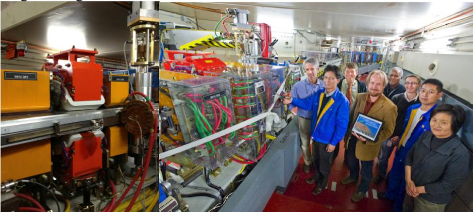
**Figure 5:** Left: SHD magnet installed between two of the QF and QD quadrupoles. Right: Ribbon cutting celebration after successful installation.
