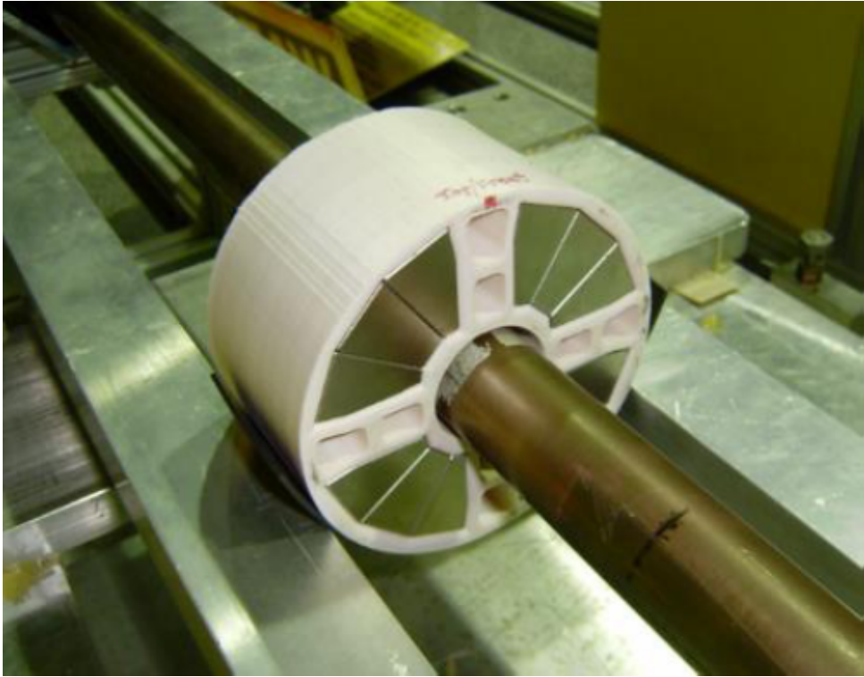
Figure 8: A modified Halbach quadrupole to avoid the synchrotron radiation, and a rotating coil device which measures the integrated multipoles of the magnet. The white material of the magnet is to hold the permanent magnet wedges together for the magnetic measurements only. The actual assembly of the magnet is different.
