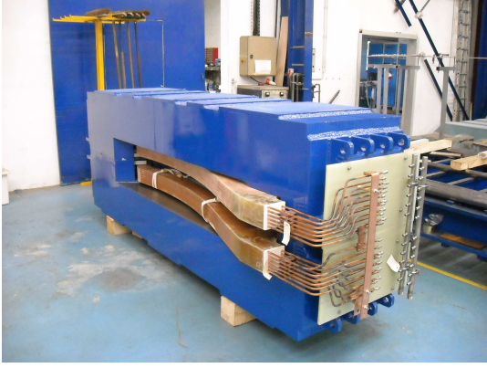
Figure 8: RACCAM spiral dipole during assembly, field clamps not yet mounted.
