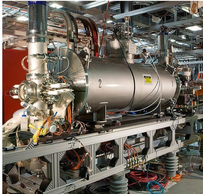
Fig. 2. RHIC EBIS before installation on BNL accelerator facility.
