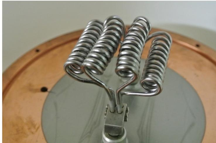
**Figure 13:** Cathode (TRF800-80) capable of producing up to 90 A at 140 V arc is made of four 2.5 mm diameter Tungsten filaments. Note the cone loss cusp lines from each filament on the back plate.
