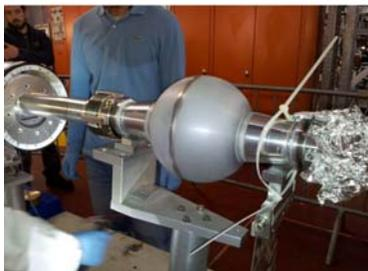
**Figure 1:** IP spherical vacuum chamber.
