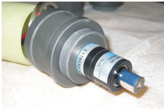
**Figure 2:** Čerenkov detector radiator and PMT
