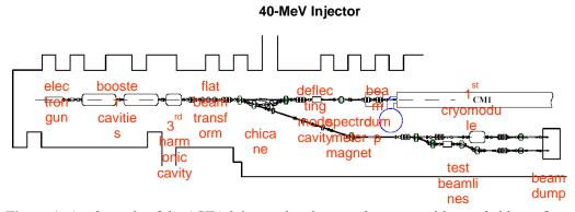
**Figure 1:** A schematic of the ASTA injector showing gun, booster cavities, and chicane for providing beam into CM1. The straight ahead line to the low energy dump is in assembly stage.
