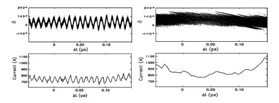
Figure 1. A 30  $\mu$ m wavelength, 1% amplitude density modulation is superimposed to an electron beam at 100 MeV. The bunch is then compressed by a factor 10, transported to the entrance of a mixing chicane (left plots) and subjected to phase mixing with  $|R_{56}|$ =30 mm. Top row: electron beam longitudinal phase space. Bottom row: current profile. Elegant code [21] particle tracking results [18].
