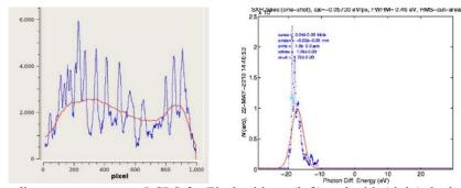
**Figure 3:** Corresponding x-ray spectra at LCLS for Fig.2 without (left) and with (right) the laser heater active [9].
