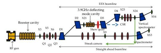
**Figure 1:** Experimental setup of the A0 photoinjector facility. Electrons generated by the RF gun are accelerated through the booster cavity to 14 MeV. Q1, Q2, Q3 focus the beam before it enters the EEX beamline. D1, D2, D3 and D4 are the dipole magnets. The skew quadrupole located before D3 is used to study time-resolved effects. X# refers to beam imaging stations.
