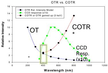
**Figure 4:** Comparison of the OTR and COTR spectral content and the CCD spectral response. The COTR gain is based on a model using the 3-keV slice energy spread [9].
