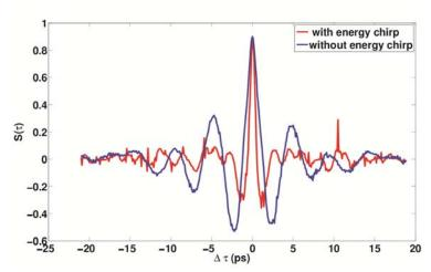
**Figure 6:** Auto-correlation measurement with Martin-Puplett interferometer with and without energy chirp.
