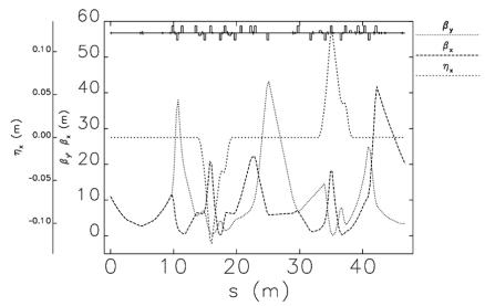
**Figure 2.** Nominal optics of the Spreader. The two MDBAs are identified by the closed dispersion bumps. The machine layout is sketched at the top.
