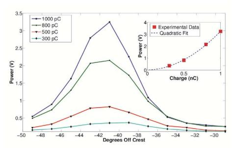
**Figure 2:** CSR Power measurement at D3 as a function of 9-cell booster cavity phase. Maximum power is observed at 41 ° off crest. The inset shows the fit of the CSR power as a function of charge.
