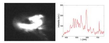
**Figure 12:** Typical COTR image (left) and wavelength spectrum following double compression at NLCTA [14].
