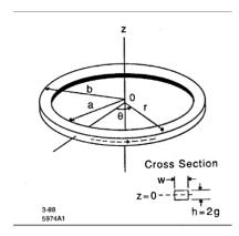
Figure 5: Toroidal chamber with rectangular cross section.
