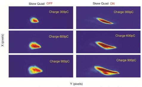
**Figure 5:** Measured transverse beam profile at X24 as a function of skew quadrupole off (left column) and skew quadrupole on (right column) for various charges. The CSR bulge effect is prominent at higher charges.
