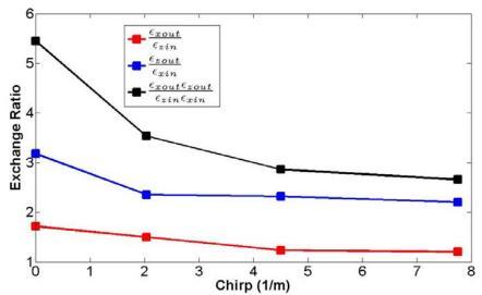
**Figure 7:** Measured value of the emittance exchange ratio and their products. As the RF-chirp increases, the ratio tends towards one. There is still some emittance dilution possibly due to second order effects and space charge.
