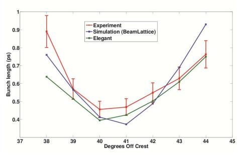
**Figure 4:** R.M.S. bunch length comparison for an \$elegant\$ simulation including CSR, a single-particle-matrix simulation without CSR, and the measurements.
