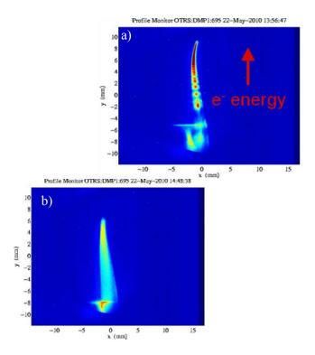
**Figure 2:** Examples of the LCLS electron beam high energy spectrum a) without and b) with the laser heater active [9].
