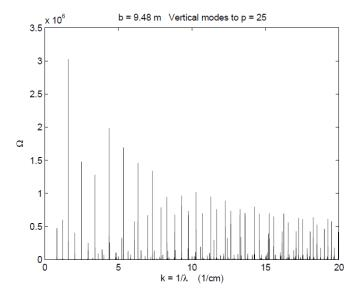
**Figure 7:** Re  $Z(n, n\omega_0)$  for parameters of VUV light source, vs. wave number  $1/\lambda$  in units of cm<sup>-1</sup>.
