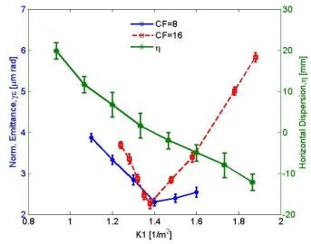
**Figure 3.** Horizontal emittance (circles for CF=8, squares for CF=16) and spurious horizontal dispersion (stars) measured at the Spreader end versus the strength of the quadrupole Q SFEL01.02 placed between the two DBAs.
