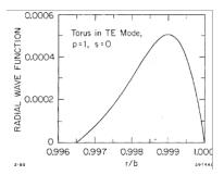
**Figure 6:** Wave functions vs. r/b for pill box and torus. Here s=0 corresponds to s=1 in the main text.
