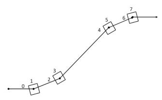
**Figure 1.** Sketch of the FERMI Spreader (not to scale). The design optics gives a betatron phase advance of  $\pi$  in the bending plane between two consecutive dipoles. There are quadrupoles between the dipoles (not shown here).
