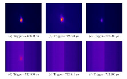
**Figure 6:** Beam images for different CCD trigger times for the chip integration period for the LYSO:Ce scintillator in (a-c) and the OTR source (d-f).
