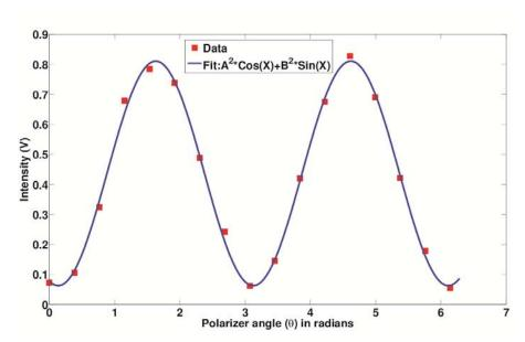
**Figure 3:** The measured CSR intensity as a function of polarizer angle. While the sinusoidal behavior indicates a horizontally polarized CSR light, the non-zero baseline indicates the vertical polarization component of the CSR. The fit function is given by  $A^2cos^2(X) + B^2sin^2(X)$  where  $X = w\theta + \phi$  and  $w, \phi, A$  and B are arbitrary constants and  $\theta$  is the polarizer angle in radians.
