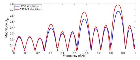
Figure 7: Magnitude of  $S_{11}$  predicted by HFSS and CST Microwave Studio (MS), for striplines with four equally-spaced Macor ring supports, and ideal 50  $\Omega$  feedthroughs.
