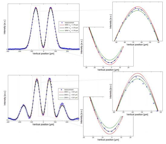
**Figure 2:** Measured (crosses) and calculated (solid lines) vertical image profiles for different beam sizes, for the new beam size monitor X08DA. The measured valley-to-peak ratio leads to the conclusion that the corresponding vertical beam size is 4.78 μm using the imaging method (top) and 4.81 μm using the interference method (bottom).
