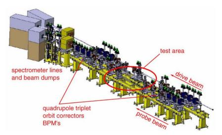
Figure 2: Two-beam Test Stand layout with the drive and probe beam lines.
