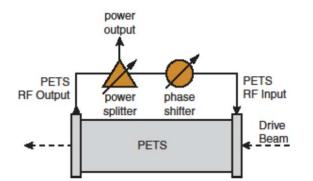
Figure 6: Layout of a PETS with external RF power recirculation option.
