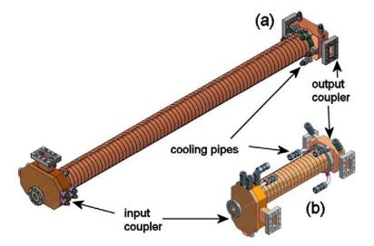
Figure 1: Mechanical drawing of the C-Band Structure (a) and prototype (b). Picture taken from [5].
