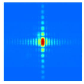
Figure 9: Interference pattern from the Mitsuhashi Interferometer at the Australian Synchrotron storage ring optical diagnostic beamline.
