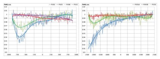
**Figure 4:** Recent in situ measurements of the longitudinal peak field profile of undulators affected by radiation damage. The lhs shows data for selected 2m IDs. PU02 and PU08 are located upstream in canted straights while PU03 and PU12 are located downstream. On the rhs data for 5m IDs are depicted. All data are normalized to values measured in the laboratory.
