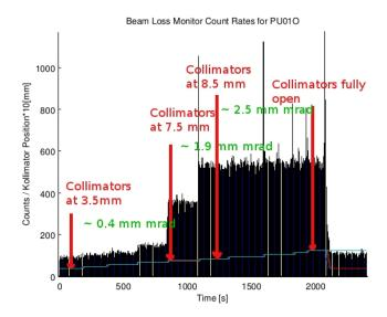
**Figure 6:** Counts measured at PIN-diode PU01(out) during top up operation with 100mA stored in 960 bunches. The set values of the collimators are varied during the measurement from nominal 3.5 mm (0.4 mm mrad) to fully open corresponding to 12 mm (4.8 mm mrad). The aperture set by the small gap undulator chamber at PU01 corresponds to 2.5 mm mrad.
