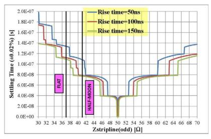
Figure 4: Settling time of the stripline voltage pulse as a function of stripline impedance for different 0% to 100% rise times of the output pulse of the inductive adder. The inductive adder, transmission line and terminating resistor impedances are 50  $\Omega$ .
