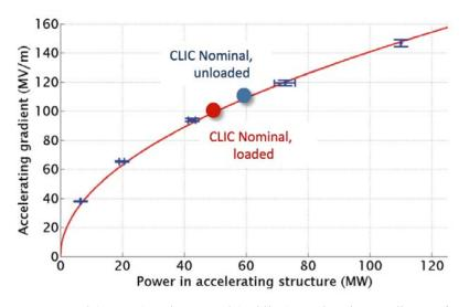
**Figure 1.15:** Measured (crosses) and expected (red line) accelerating gradient as function of the RF input power for accelerating structure TD24\_vg1.8 used in the 2011 run. The Nominal CLIC conditions (100 MV/m loaded and 110 MV/m unloaded) are also reported.
