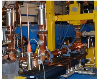
Figure 3: First C-Band structure under high power test in the SPARC experimental hall.
