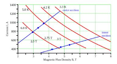
Figure 4: Load lines of the inner and outer coil sections (blue) and critical current as a function of magnetic flux density and temperature (red)
