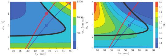
**Figure 1:** (a) Normalized equilibrium horizontal emittance as a function of wiggler period lenght and flux density amplitude. The solid black line indicates the target normalized emittance for the CLIC damping rings. The blue and red line indicate the maximum achievable operational flux density amplitude as a function of period length for a magnetic gap of 18 mm for Nb-Ti and Nb<sub>3</sub>Sn technology, repectively. (b) Ratio of normalized emittance including intra beam
