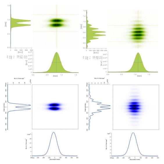
Figure 7: Measured image intensity (upper) and simulated image intensity (lower) during nominal user operation, for 325 nm wavelength using the imaging method (left) and the interference method with a 25 mm horizontal obstacle (right).
