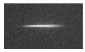
Figure 8: Image of the OTR PSF measured at ATF2 using vertically polarised photons.
