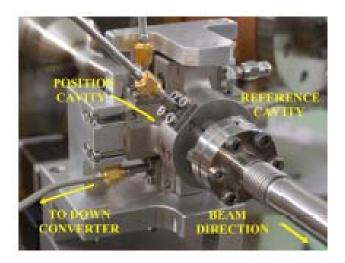
Figure 1:. Prototype cavity BPM installed in TBTS.
