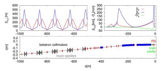
Figure 1: Optics (top) and layout (bottom) of the CLIC betatron collimation and FF sections.
