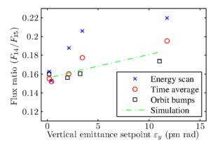
Figure 13: Comparison of the flux ratio measurements for the range of set vertical emittances using various techniques to take the flux data.
