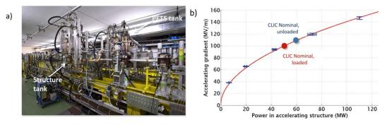
**Figure 2:** a) The Two-Beam Test Stand at the CLIC Test Facility where 12 GHz rf power is extracted from an up to 28 A drive beam and transferred to structure accelerating a 1 A probe beam. b) Experimental results of two-beam acceleration, up to and beyond the nominal CLIC gradient.
