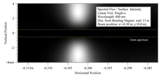
Figure 7: Simulated SR distribution on target.
