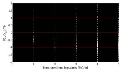
Figure 4: Mode spectrum of the vertical coherent motion for positive chromaticity.
