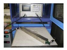
Figure 5: Measurements setup: network analyzer, the transmission coefficient S<sub>21</sub> of an X-band waveguide is measured.
