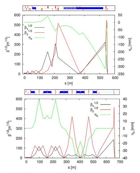
Figure 9: Optics of the CLIC 500 GeV local correction scheme (top) and dedicated correction scheme (bottom) final focus system showing horizontal and vertical beta-functions.
