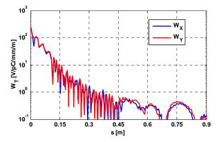
Figure 9: The envelope of the transverse wakefields for both planes is shown. The CLIC bunch spacing is 0.15 m.
