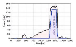
Figure 3: Typical RF pulse shape in ASTA. Here, for convenience, we also have plotted the shape of the CLIC target pulse.
