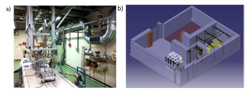
**Figure 9:** a) The new X-band test facility at CERN, with a SLAC-procured 12 GHz klystron. b) A planned X-band test facilities which will include commercially acquired tubes from CPI and Toshiba. In total these facilities will provide X-band power for testing up to 8 accelerating structures simultaneously.
