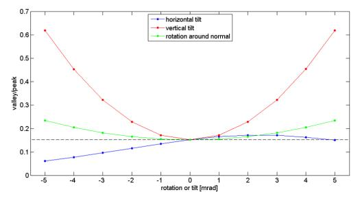
Figure 6: Calculated valley-to-peak ratio (VPR) as a function of the different misalignments.
