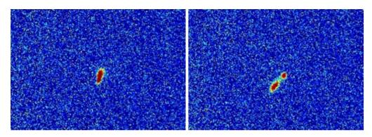
**Figure 12:** Example of a double beam spot detected on a beam screen in correspondence of a RF breakdown in the accelerating structure (right) and the beam under normal operating conditions (left). The image on the right is interpreted as one part of the beam pulse having received a kick during an RF breakdown event.
