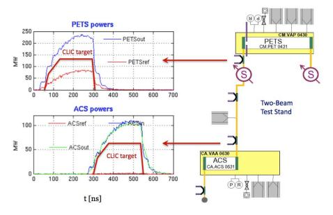
**Figure 1.11:** RF signals measured in different locations of the TBTS. The use of recirculation allowed to reach in the PETS (above) and in the accelerating structure (below) RF power levels and pulse lengths well beyond the CLIC nominal value.
