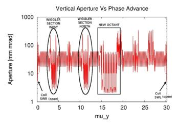
**Figure 5:** Normalized vertical aperture in PETRA III. Small vertical apertures are set by absorbers in the wiggler sections west and north and by the small gap chambers at the IDs in the new octant. The movable vertical collimators are closed down to ~0.4 mm mrad during user operation.
