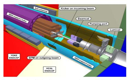
Figure 4: Interaction region showing the QD0 support tube surrounded by the anti-solenoid and all the other elements down to the Lumical.
