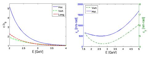
Figure 3: Dependence of the IBS growth factor, i.e. ratio between steady state and equilibrium emittances (left) and steady state emittances (right) with energy.
