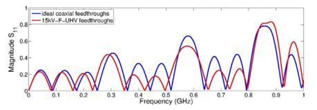
Figure 9: Predicted magnitude of  $S_{11}$  for striplines with ideal coaxial feedthroughs and with Kyocera 15kV-F-UHV feedthroughs.
