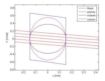
Figure 1: Horizontal phase space diagram of a pinhole array showing the overlap of the pinhole phase space with the x-ray and electron beam phase space.
