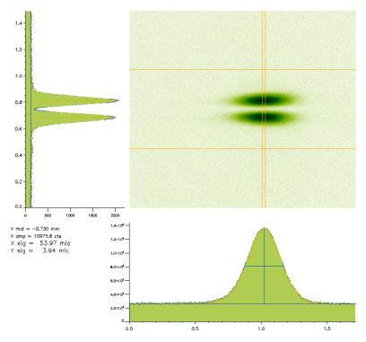
Figure 9: Screen shot of smallest vertical beam size of  $\sigma_y \sim 4 \mu m$  measured so far with the SLS X08DA beam size monitor using the  $\pi$ -polarization imaging method.
