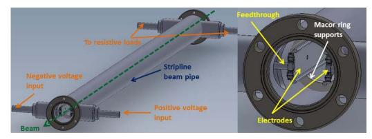
Figure 1: 3D model of a stripline kicker.
