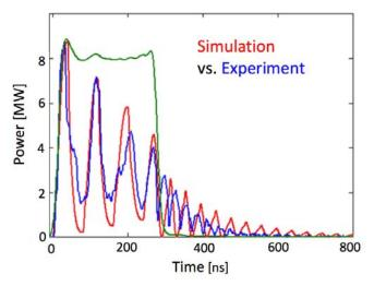
Figure 1.13: The simulated (red) and measured (blue) RF pulses generated by PETS in the Off state. The direct power production (On state) is shown in green.
