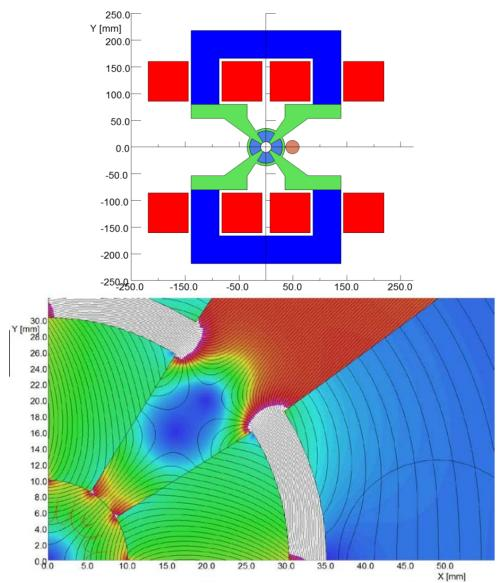
**Figure 8**: QDO design based on hybrid technology proposed for the ILC FFS [10]. The top figure shows a transverse section of the design and the bottom plot shows the field lines in the main beam pipe and the aperture for the extracted beam.
