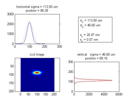
Figure 8: Beam profiles from direct visible light imaging with an f = 3.5 m focal length achromatic focussing lens and an optical aperture that reduces the diffraction from the frontend mask and the mirror edge.
