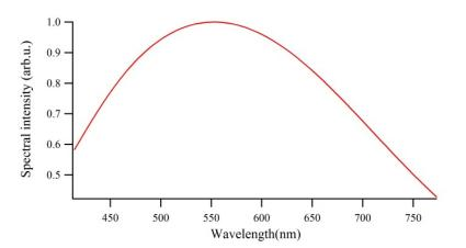
Figure 13: Spectrum of SR emitted with angle 2-3 mrad from a 500 MeV electron beam crossing an undulator with 3 periods, K=1.3,  $\lambda_u$ =12 cm. Simulated with SRW.
