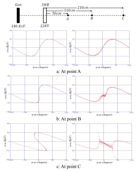
Figure 9: The phase space of the beam at several distances away from SHB ignoring the space charge (left diagram) and taking it into account (right diagram).
