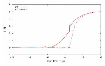
Figure 12: The longitudinal field of the experimental solenoid along the beamline, with and without anti-solenoid.
