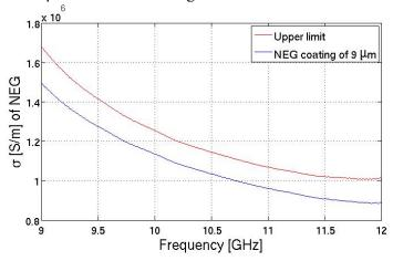
Figure 6: Conductivity of NEG as a function of frequency.
