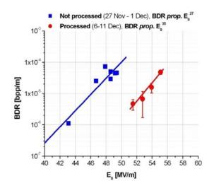
**Figure 2:** Breakdown rates as measured at different field values before and after conditioning of the SPARC C-Band prototype (plots taken from [5]). After processing, about 50MV/m accelerating field has been reached, with a breakdown rate per meter of the order of 10<sup>-6</sup>.
