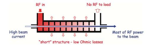
Figure 1.3: Acceleration of a beam in a travelling wave structure. Under full beam loading operation no RF power is leaving the structure.
