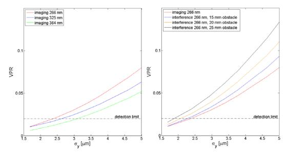
Figure 3: Calculated valley-to-peak ratio (VPR) as a function of the rms vertical beam size for different wavelengths (left) and for different measurement methods (right).
