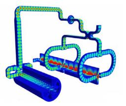
Figure 1: Electric filed plot in the CLIC two-beam accelerator unit. Here the PETS (shown left) is driven by the steady state drive beam current (courtesy SLAC).
