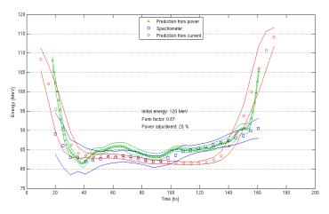
**Figure 1.17:** Comparison between the measured time resolved energy profile of the beam along the pulse with a segmented beam dump and the predictions from beam current and power production measurements. The data points shown are the average of 48 consecutive pulse and the shaded areas indicate the standard deviation for the measurement over this pulses.
