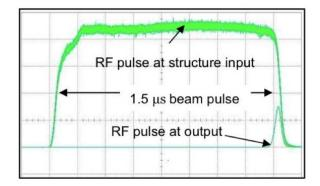
Figure 1.4: RF power measured at the accelerating structure input and output with beam.
