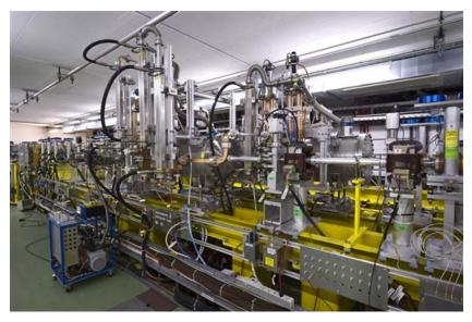
Figure 4: Photo of the TBTS experiment area with vacuum tanks for PETS (to theright) and accelerating structure (at the left) [19].
