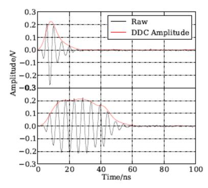
Figure 2: Example of digitised signals from the cavity BPM as excited by a short beam pulse (top) and long beam pulse (bottom) with the amplitude as measured using digital down-conversion.
