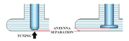
Figure 3: Waveguide to coaxial transition in the first prototype (left) and the new design with a bead on the antenna tip (right).
