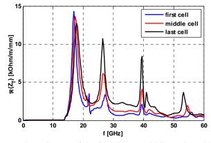
Figure 8: Transverse impedances of the first (blue), middle (red) and last (black) cells.
