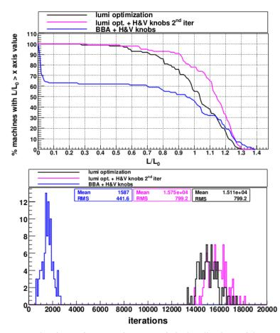
**Figure 3**: Top: Luminosity performance for 100 statistical realizations of the CLIC FFS after tuning using 3 different approaches. Bottom: Required number of luminosity measurements for the 3 different approaches.
