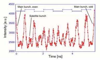
Figure 1.2: Fast bunch phase switch, measured in CTF3 by a streak camera.
