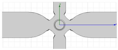
Figure 5: Internal volume of the coupler cell.
