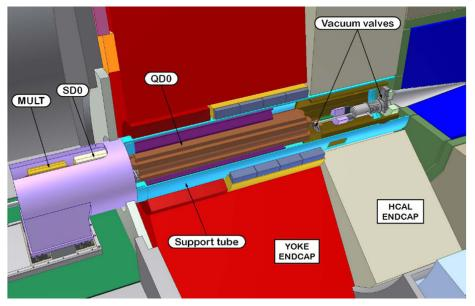
Figure 1: CLIC Machine Detector Interface layout (configuration for 3 TeV machine energy with L\* of 3.5 m).
