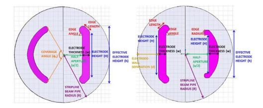
**Figure 2:** Schematic of the geometric parameters, for a curved and a flat electrode (left), and t for a flat and a half-moon electrode (right).
