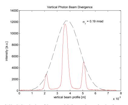
Figure 3: Vertical projection of the x-ray pinhole array image showing the natural opening angle of the dipole radiation.
