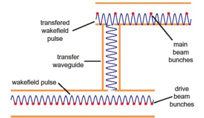
**Figure 1:** Two-beam acceleration scheme. The RF wakefield created by the drive beam is transferred to the main (probe) beam accelerating structures. Due to differences in the group velocity of the RF wave, the energy density is increased and thereby the electric field magnitude.
