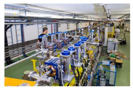
Figure 3: Photo of the Two-beam Test Stand with the drive beam line (left) and probe beam line (right) [18] before installation of PETS and accelerating structure.
