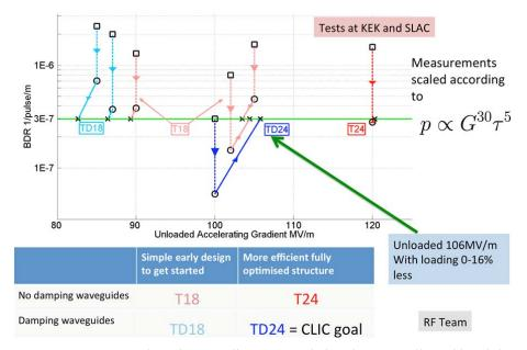
Figure 3: Structure test results, where gradients are scaled to the CLIC allowed breakdown rate of  $3 \times 10^{-7}$ . A fully optimized CLIC structure with damping waveguides has recently reached an unloaded gradient of 106 MV/m.
