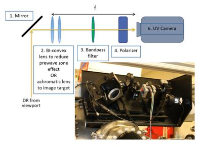
Figure 3: Schematic and image of the optical system.
