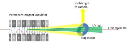
Figure 10: Schematic of off-axis SR observation.
