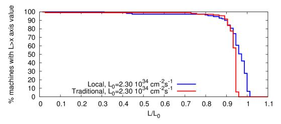
Figure 11: Luminosity distribution of 100 machines after BBA and multiknob algorithm procedure for an initial prealignment of 10 microns
