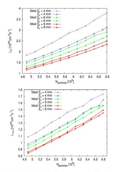
Figure 7: Total (top) and peak (bottom) luminosity versus number of particles per bunch and for 3 different IP horizontal beta functions using ideal distributions and new FFS designs. The vertical beta function has been set to the minimum value allowed by the hourglass effect (0.065mm).
