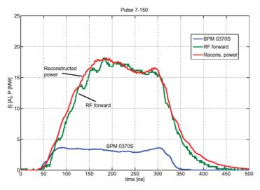
**Figure 7:** Example of a drive beam pulse with measured (marked RF forward) and reconstructed RF power generation from the PETS. RF recirculation gain g = 0.75 and phase shift  $\phi = 18^{\circ}$ . Recirculation round-trip time  $\tau = 26$  ns. For comparison, the BPM pulse is also shown.
