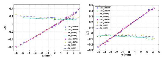
**Figure 4:** Dependency of the difference-over-sum ratio on the beam displacement in the horizontal (Left) and vertical (Right) plane for PETS RF power values of 6 MW (dashed lines) and 60 MW (solid lines).
