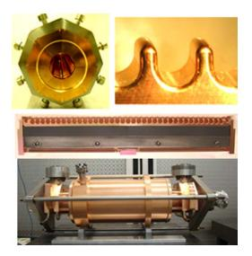
**Figure 2:** The front view of the assembled PETS body (top left), zoom of the PETS single bar period (top right), the single bar equipped with damping loads (centre) and fully assembled structure (bottom).
