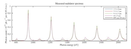
Figure 11: Measured undulator spectrum in vertical polarisation mode on the soft x-ray beamline at the Australian Synchrotron.
