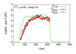
**Figure 9:** Measured with the spectrometer the drive beam deceleration (black line) and the one calculated from power measurements (red line) are shown together with the pulse current (green line). It shows the same pulse as in Fig. 8.
