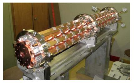
**Figure 1.10:** The 12 GHz PETS prototype installed in the TBTS. The PETS is based on the CLIC baseline design but longer (one meter as opposed to 0.21 m for CLIC) in order to reach and exceed the CLIC nominal power in spite of the lower CTF3 Drive Beam current (30 A maximum, as opposed to 100 A for CLIC).
