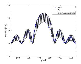
Figure 10: Intensity imbalance interferometer pattern where the visibility has been reduced in a controlled way to reduce the error in the measurement.
