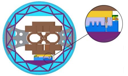
Figure 11: The supporting concept of the full-size QD0 inside the experiment detector.
