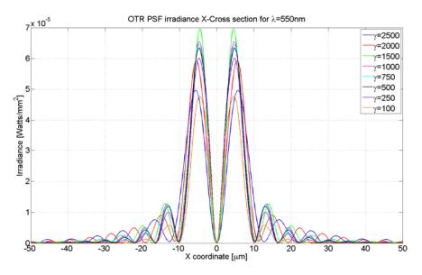
Figure 7: Horizontal cross-section of the OTR electric field distribution calculated for different beam energies.
