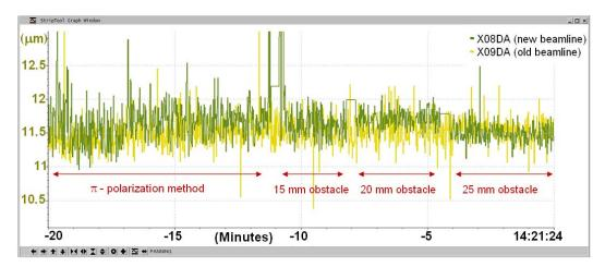
**Figure 8:** Comparison of the vertical beam sizes measured simultaneously with the old and the new beam size monitor, which are located at ring positions with identical beta functions. The measurements on the new beam size monitor are done with the imaging and the interference measurement methods using different obstacle sizes.
