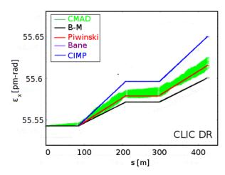
Figure 6: The one turn behaviour of the horizontal emittance starting from the zero current values, as computed by CMAD-IBSTrack (green), BM (black), modified Piwinski (red), Bane (purple) and CIMP (blue) formalisms.
