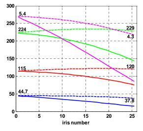
**Figure 7:** The fundamental mode properties are shown in the regular cells. The traces from top to bottom are:  $S_c \cdot 50 \, [W/\mu m^2]$ (pink), surface electric field [MV/m](green), accelerating gradient [MV/m](red), pulse surface temperature rise [K](blue). Dashed traces are unloaded and solid are beam loaded conditions.
