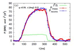
**Figure 8:** Measured RF pulse (red line) and reconstructed signal (blue line) are shown together with the current pulse used as an input for reconstruction (green line).
