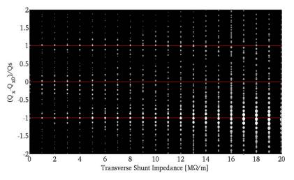
Figure 3: Mode spectrum of the horizontal coherent motion for positive chromaticity.
