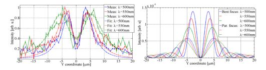
**Figure 9:** A comparison between the measured (left) and simulated (right) PSF for 500nm, 550nm and 600nm wavelengths.
