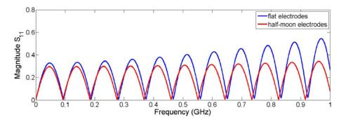
Figure 3: S<sub>11</sub> for flat electrodes (blue) and half-moon electrodes (red), for a frequency range from DC to 1 GHz.
