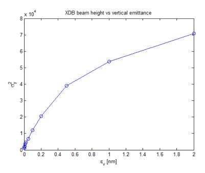
Figure 6: Square of the vertical beam size plotted against a calculated emittance coupling using the calibrated LOCO model using an emittance minimisation process.
