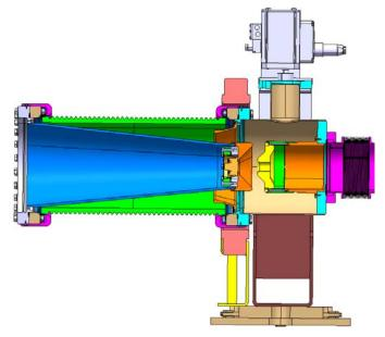
Figure 1: Conceptual design of the drive beam gun. Ceramic isolator (green), Anode (yellow), Focusing electrode (orange), cathode (light orange).
