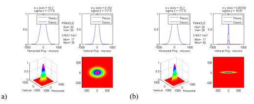
Figure 4: Effective point spread function for pinhole camera and YAG screen system for (a) nominal 1% and (b) minimised 0.01% emittance coupling.
