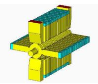
Figure 2: 12 cell crab cavity design including wakefield dampers (length of 300 mm).
