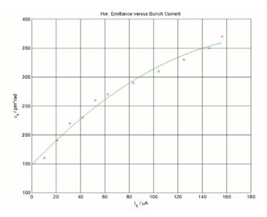
Figure 3: Horizontal emittance versus the single bunch current of PETRA III at 3 GeV.
