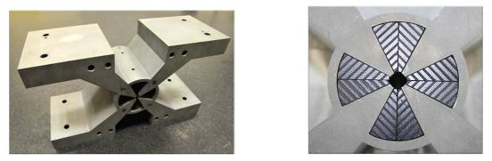
Figure 6: The prototype core elements: the monolithic Permendur structure (left) and a details of the PM wedges inserted in the central part (right). The lines on the PM surface indicate the magnetization directions.
