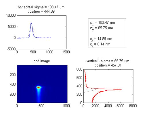
Figure 7: Initial images from the optical diagnostic beamline before correcting diffraction effects from the front end mask and the extraction mirror.
