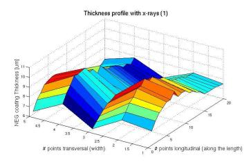
Figure 7: NEG coating profile of the Cu waveguide with x-rays fluorescence.
