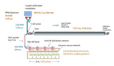
Figure 5: An rf unit for a klystron based CLIC. Two 60 MW klystrons can power 8 CLIC accelerating structures at a gradient of 100 MV/m.
