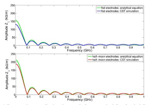
**Figure 6:** Transverse beam coupling impedance results for untapered striplines from both Eq. 2 (green) and CST PS simulations for flat electrodes (blue) and half-moon electrodes (red).
