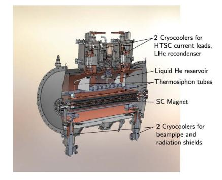
Figure 5: Cross section of the CLIC damping wiggler prototype (graphics from [13])
