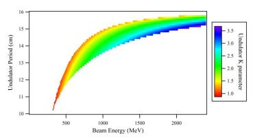
Figure 11: Undulator period and K parameter needed to produce 500 nm light at an opening angle of 2.5 mrad for different beam energies.
