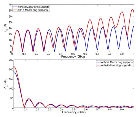
**Figure 8:** Longitudinal (top) and transverse (bottom) beam coupling impedance for striplines with and without Macor rings, simulated with CST PS, for ideal 50  $\Omega$  feedthroughs.
