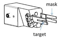
Figure 6: Target holder with mask and target mounted.
