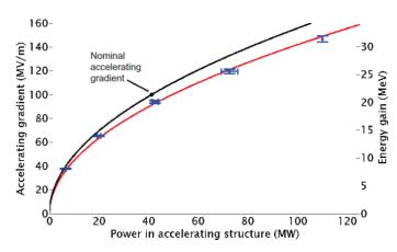
Figure 9: Measured and nominal (upper line) accelerating gradient as function of the RF input power for accelerating structure 12WDSDVG1.8 (2011 run). The corresponding beam energy gain is given on the right hand axis.
