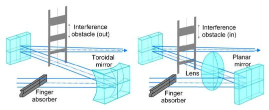
**Figure 5:** Schematic view of the X08DA beam line central region in final and intermediate configurations, using a toroidal mirror (left) and a lens with planar mirror (right). The measurement method is defined by the position of the interference obstacle; in the imaging method the obstacle is out of the beam path (left), in the interference method the obstacle obstructs the center of the beam (right).
