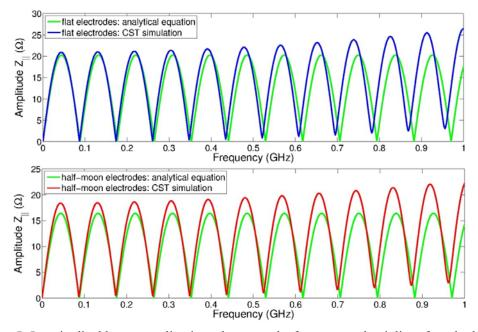
**Figure 5:** Longitudinal beam coupling impedance results for untapered striplines from both Eq.1 (green) and CST PS simulations for flat electrodes (blue) and half-moon electrodes (red).
