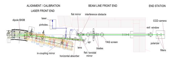
Figure 4: Layout of the X08DA beam line, laser front end and end station are schematic.
