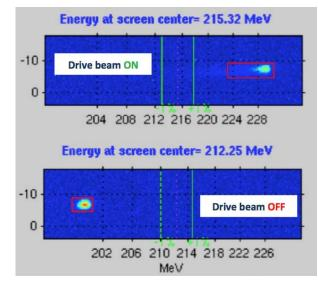
**Figure 1.14:** Probe Beam observed in the TBTS spectrometer screen with the 12 GHz RF power from the drive beam on (top) and off (bottom). The energy gain is about 31 MeV which corresponds to a gradient of 145 MV/m in the accelerating structure.
