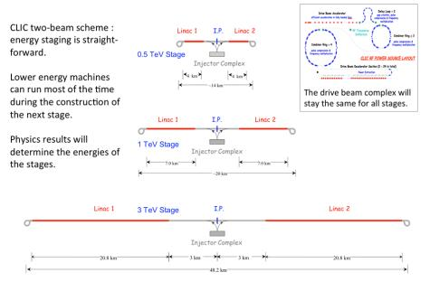
Figure 4: Example of CLIC energy stages. The center of mass energy can be increased without modifications to the drive beam accelerator complex. The actual energy of each stage will be guided by LHC physics results.
