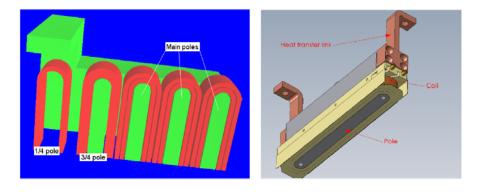
Figure 3: Octant of a short wiggler model (left), main poles with two coil sections each and 3/4-1/4 matching poles; 3D model of a single coil with extended iron core and heat transfer links (right), graphics from [13]
