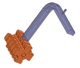
Figure 10: Geometry of one of the four arms of the wakefield monitor. (Courtesy of F. Peauger, CEA, France).
