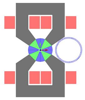
Figure 3: Two PM Halbach tunable quadrupole.
