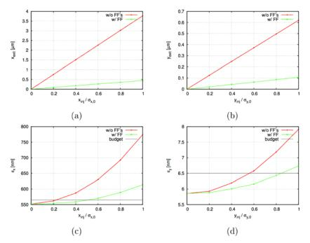
**Figure 4:** Plots of the orbit jitter (a, b) and normalised emittance (c, d) at the exit of the RTML versus orbit jitter at the entrance of the RTML in the horizontal and vertical planes respectively.
