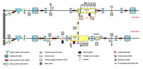
Figure 5: Layout of the two beam lines and installed equipment. The drive beam is the upper line, the probe beam is the bottom line.
