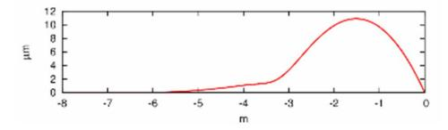
Figure 13: The vertical orbit distortion due to the solenoid field.
