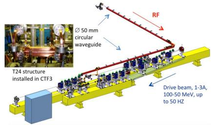
**Figure 7:** A new beam loading test facility: a 1 A CTF3 beam and X-band rf power will be simultaneously delivered to an accelerating structure.
