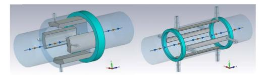
Figure 5: Initial (left) and modified (right) stripline BPM prototypes for CLIC DB.
