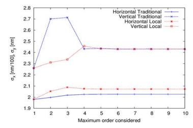
Figure 10: High order optimization using MAPCLASS for CLIC 500 GeV FFS.
