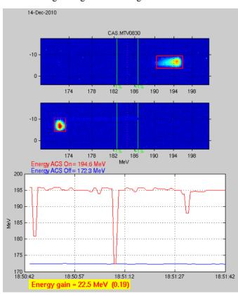
Figure 10: Two-beam acceleration measurement of the probe beam. The probe beam is operated at double repetition frequency compared to the drive beam and RF power pulse. Thus every other pulse is accelerated (top beam profile monitor snap-shot) while the pulse in between is not (bottom beam profile snap-shot). The bottom graph shows the stability of the probe beam energy with (ACS on, upper line) and without acceleration (ACS off, lower line).
