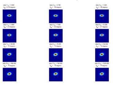
Figure 5: X-ray pinhole beam axis title measurement for a range of emittance coupling settings.
