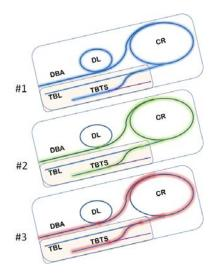
**Figure 4:** The drive beam generation modes in CTF3: 1– with full recombination (×8), 2 – with partial recombination (×4), and 3 – without recombination.
