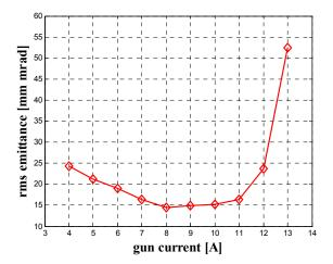
Figure 2: RMS emittance as a function of beam current for a fixed geometry.
