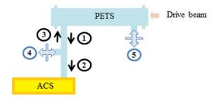
**Figure 12:** Layout of the PETS ON/OF setup in TBTS. The black arrows show RF power flows in the system: 1) RF power extracted from the PETS; 2) RF power transmitted to the accelerating structure; 3) RF power reflected back into the PETS. The new components are: 4) variable RF reflector; 5) variable RF short circuit.
