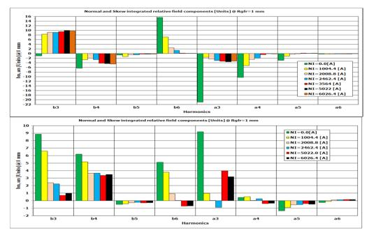
Figure 9: Field quality measurements as multipole content.
