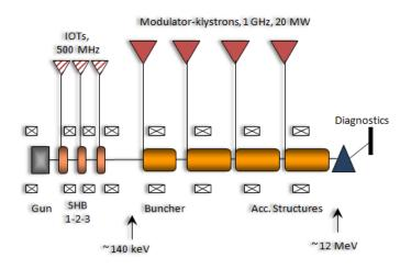
Figure 1: CLIC drive beam front-end layout.
