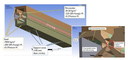
Figure 10: The full-size QD0 as a modular assembly of shorther sections.
