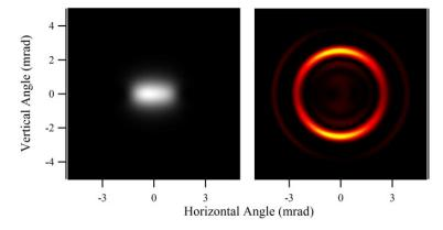
Figure 12: Total SR (left) and visible SR (right) from a 500 MeV electron beam crossing an undulator with 3 periods, K=1.3,  $\lambda_u$ =12 cm. Simulated with SRW.
