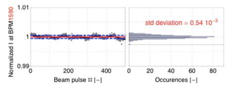
Figure 1.6: Beam current fluctuations measured at the end of the CTF3 linac.
