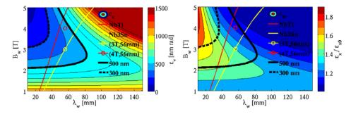
**Figure 5:** Dependence of the steady state emittance (left) and its ratio with the equilibrium emittance (right) as a function of the wiggler peak field and period. The blue color denote smaller emittances or ratios, whereas the red ones bigger. The black curve traces the horizontal emittance target barrier of 500nm.
