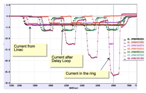
Figure 1.5: Beam current multiplication in CTF3.
