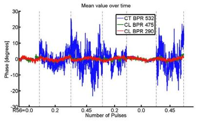
**Figure 1.8:** Mean phase value vs. time measured before the stretching chicane red and green traces) and after it (blue trace). The phase is measured in 12 GHz degrees, and the different  $R_{56}$  values used in the chicane during the measurement are indicated on the horizontal axis. For  $R_{56}$ = 0 the phase jitter is very close in all positions, and its rms is below 2°.
