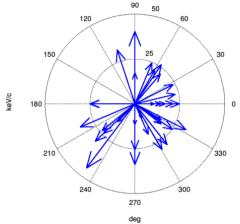
Figure 13: Compass plot showing direction and transverse momentum of beam trajectory kicks in correspondence to a RF breakdown in the accelerator structure. The transverse momentum is calculated considering the beam energy and the distance between the screen used for the measurement and the accelerator structure.
