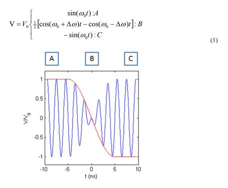
Figure 2: Smooth 180° phase switching model.
