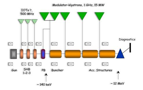
Figure 2: Schematics of the CLIC drive beam injector front end.
