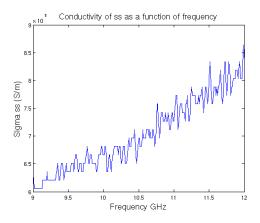
Figure 8: StSt conductivity as a function of frequency.
