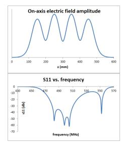
**Figure 5:** On-axis electric field amplitude and s<sub>11</sub> with a tuned coupler.
