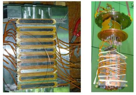
Figure 6: Short model coil assembly (left) and experimental set-up for the quench and cooling performance tests (right), photographs from [13]
