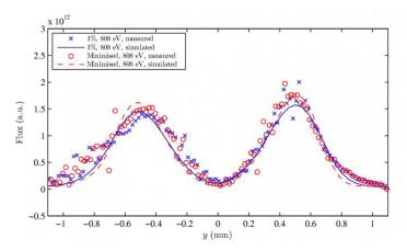
**Figure 12:** Vertical blade scan across the vertical undulator radiation at an even harmonic for 1% emittance coupling and for minimum emittance coupling (modelled to be 0.5 pm rad).
