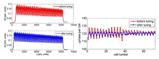
Figure 4: Measured field and phase advance per cell before and after the tuning.
