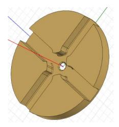
Figure 1: Basic cell geometry of the accelerating structure with strong waveguide HOM damping is shown.
