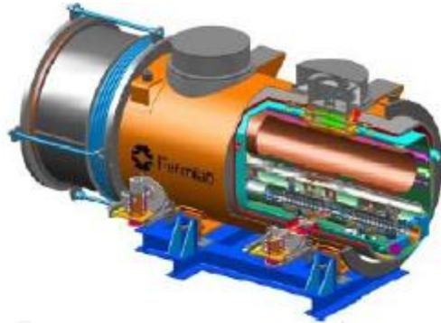
**Figure 1:** Schematic of a FNAL cryo-module [4] consisting of four 3.9 GHz cavities.
