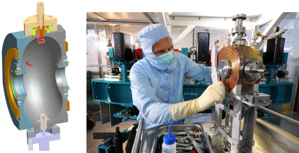
**Figure 4:** Design of an EMMA RF cavity (left) and a cavity under test (right).
