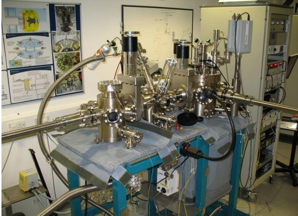
**Figure 7:** The assembled photocathode preparation facility.
