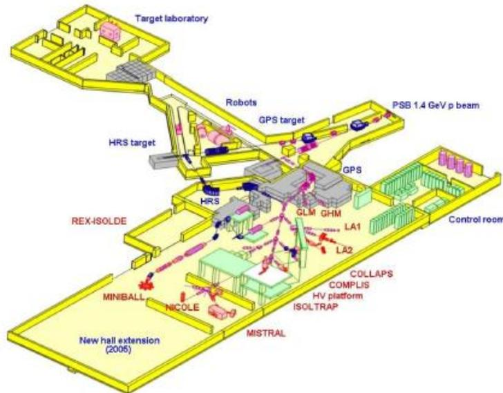
**Figure 1:** Schematic of the ISOLDE facility at CERN, showing the existing hall extension that is allocated to the new accelerator HIE-LINAC.
