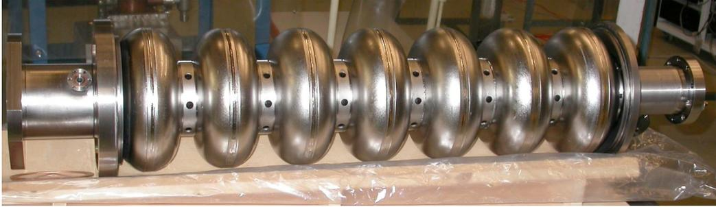
**Figure 3:** 7-cell cavity after final electron-beam welding.
