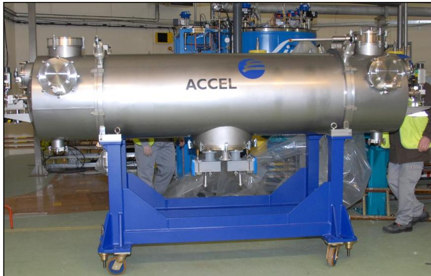
**Figure 1:** ACCEL ERL cryomodule preparing to be installed on ALICE.
