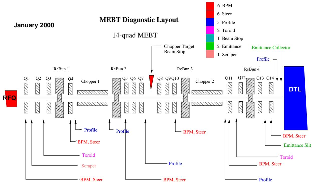
Figure 3.8: MEBT logical layout and diagnostics complement
