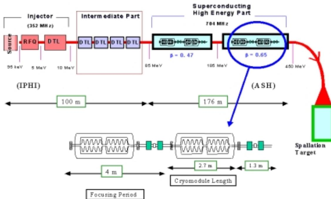
Figure 3.34: Layout of a High Power Proton Accelerator
