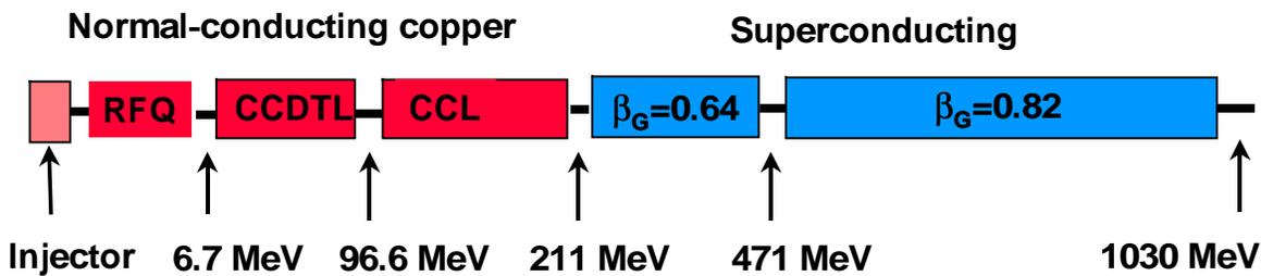
Figure 3.17: Block diagram of the APT linac.
