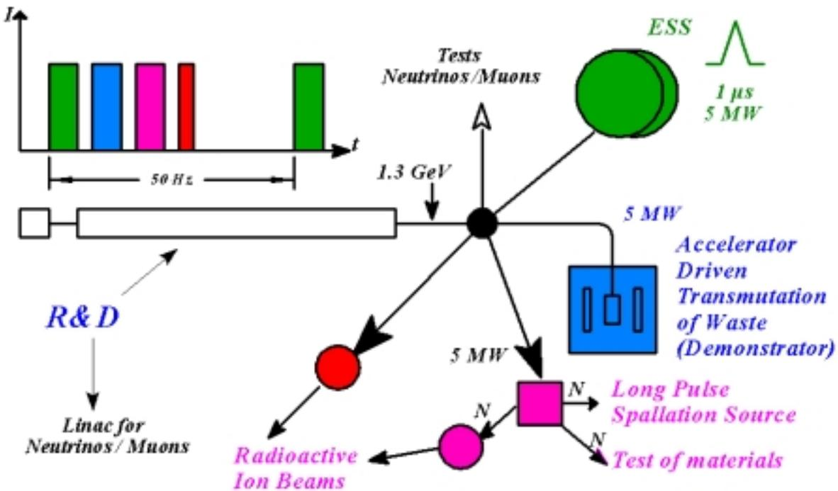
Figure 3.35: Schematic layout of a multi-application facility using a high-power proton accelerator.)
