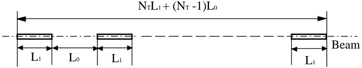
Figure 5.4: The layout of the aligned tubes in a laser-wakefield accelerator.
