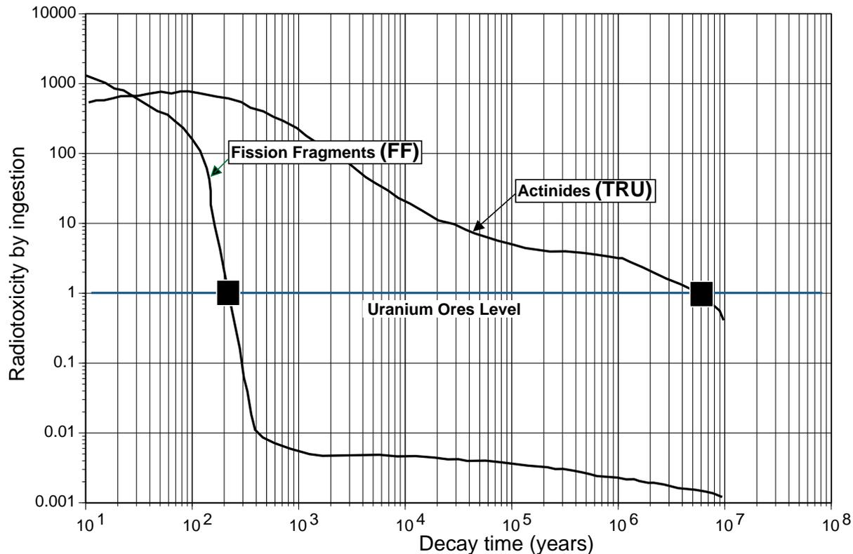
Figure 3.18: Time evolution of the potential radiotoxicity (relative to uranium ore) of the two main components of nuclear waste for PWR spent fuel, obtained with the ORIGEN2 code.
