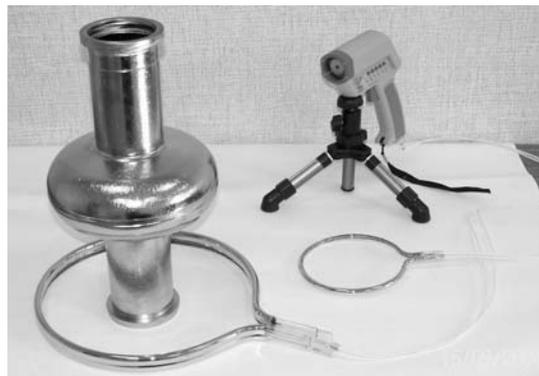
**Figure 14:** 1.3 GHz cavity, IR heaters and thermal sensor used in “fast baking” experiment
