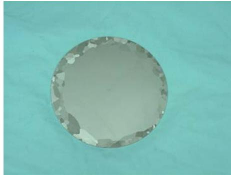
**Figure 6:** Large grain niobium sheet for cavity fabrication; the center represents a single crystal.
