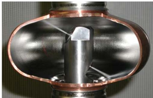
**Figure 9:** Test of the CO<sub>2</sub>-snow nozzle system in a cut NbCu cavity.
