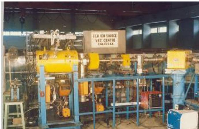
**Figure 2:** The 6.4 GHz ECR ion source and the initial portion of injection line together with the charge state analyser.
