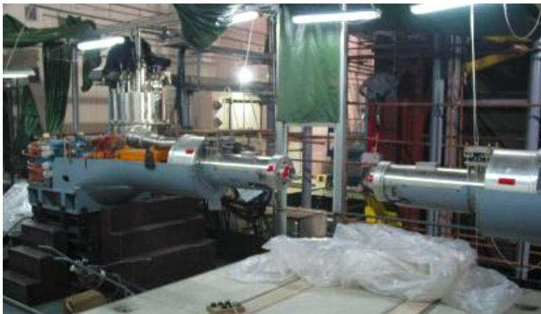
**Figure 7:** SCQ's and some warm magnets installed in IR
