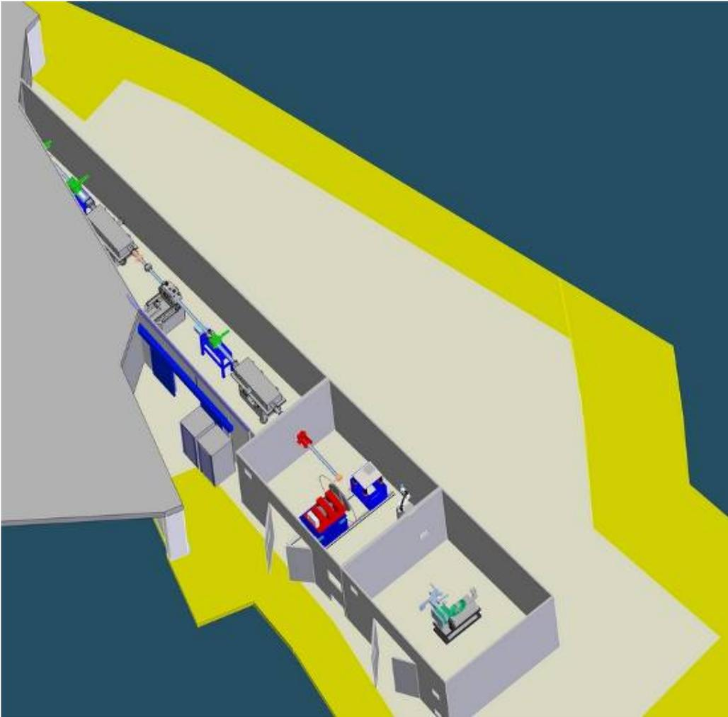
**Figure 5:** Cut-away layout of one of the Powder Diffraction Beamline, showing the optical components housed in the first hutch, followed by two experimental hutches.
