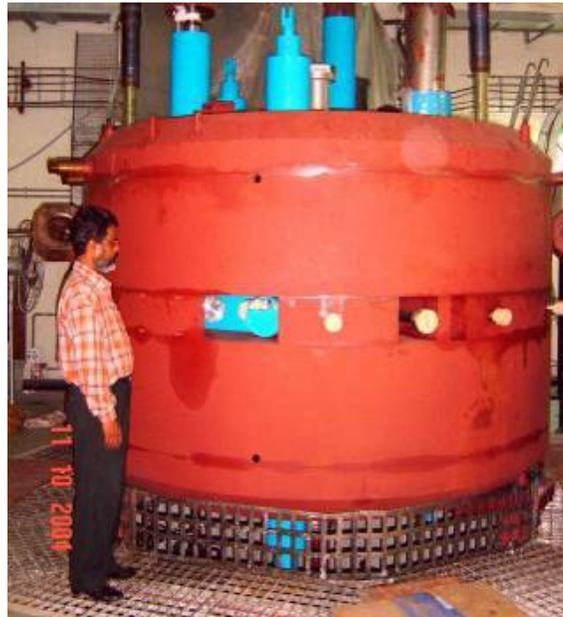
**Figure 5:** 80 tonne cyclotron magnet with cryostat installed in it.
