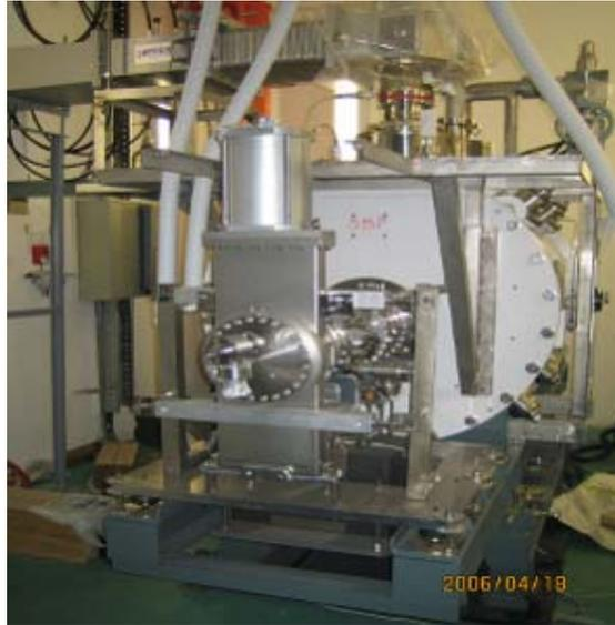
**Figure 3:** A RF cavity in test
