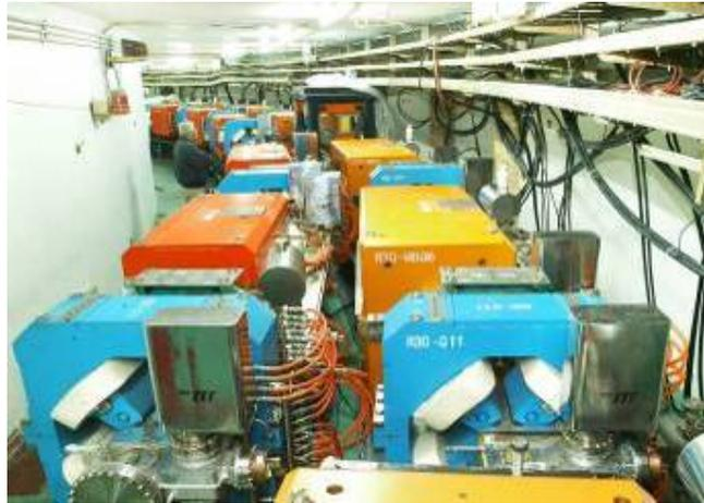
**Figure 8:** Installed accelerator units in the BEPCII tunnel
