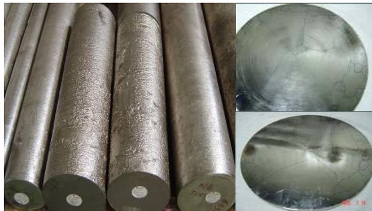
**Figure 11:** Chinese Ning Xia large grain Nb. Left – RRR300 Grade Nb Ingot; right – Slices of RRR300 Ingot.
