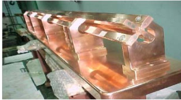
**Figure 9:** A half-scale model of the RFQ with un-modulated vanes.
