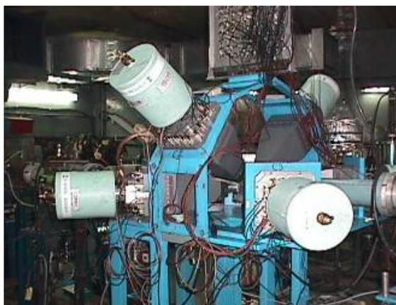
**Figure 3:** The Indian National Gamma Array setup in Ch#3 using clover detectors.
