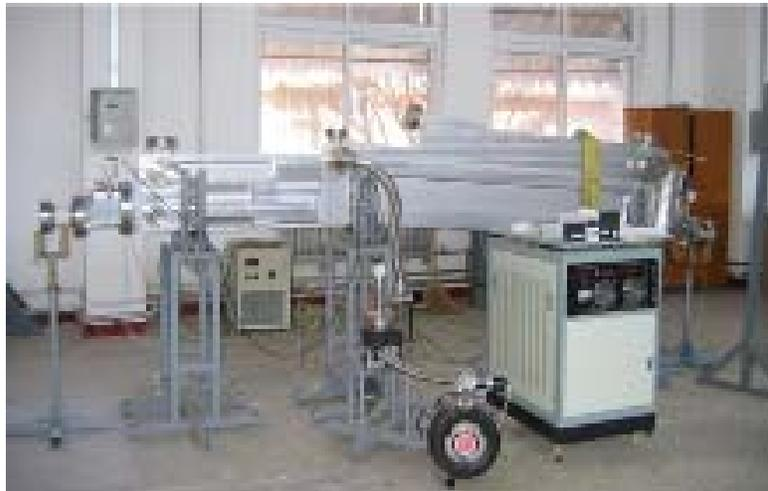
**Figure 6:** An aluminium antichamber in coating
