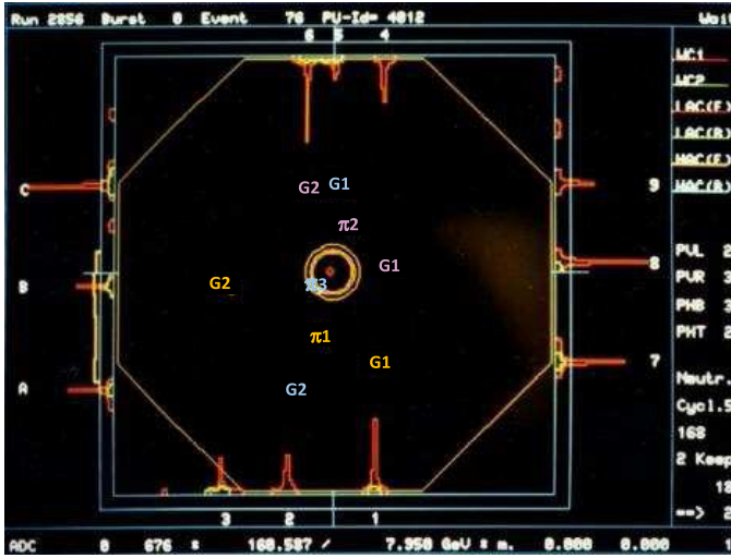
Fig. 2. Display of a 3\pi^0 candidate event. On the borders of the squared area representing the LAC surface are drawn peaks corresponding to the energy deposition in the horizontal and vertical calorimeter strips. The reconstructed photon positions are denoted by the letters G_j . The positions of the three \pi^0 are indicated by \pi_i . Different colours are used for each \pi^0 and its decay products.
