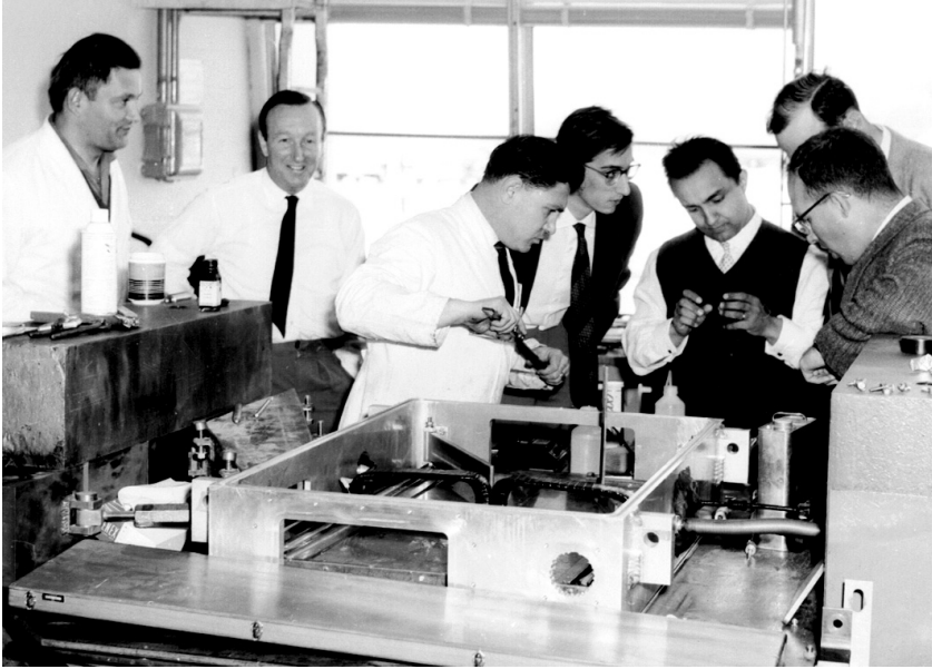
Fig. 1. First experimental magnet in which muons were stored at CERN for up to 30 turns. Left-to-right: Georges Charpak, Francis Farley, Bruno Nicolai, Hans Sens, Antonino Zichichi, Carl York, Richard Garwin.
